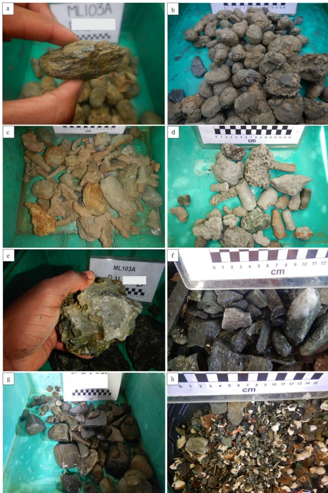
Figure. 5.8. Drill core screens showing a) Saprolite b) Mudballs c-d) Sandstone tubes formed by reef-building tubeworms, Diplochaetetes longitubus . e) Traces of of Diplochaetetes longitubus bioturbation in sandstone. f) Lower gravel beach material. g) Middle gravel beach material with abundant banded ironstone clasts. h) Upper gravel beach material containing shell hash and finer gravels.
