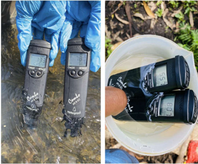
Figure 3.12 Measurements of the hydrochemistry parameters (EC, temperature and pH) using the Waterproof Portable Meter. (a) immersed directly into a stream, (b) immersed in a beaker.
