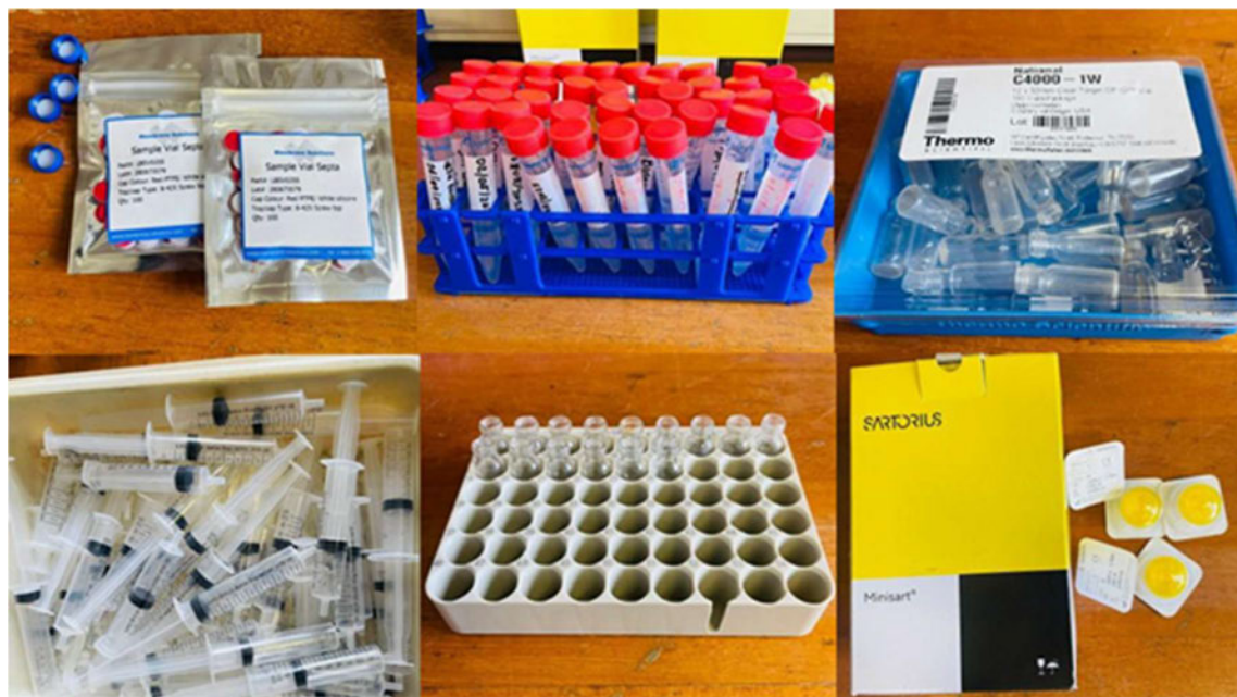
Figure 3.13 Apparatus used to collect and filter samples in preparation for ^2\text{H} and ^{18}\text{O} analysis.
