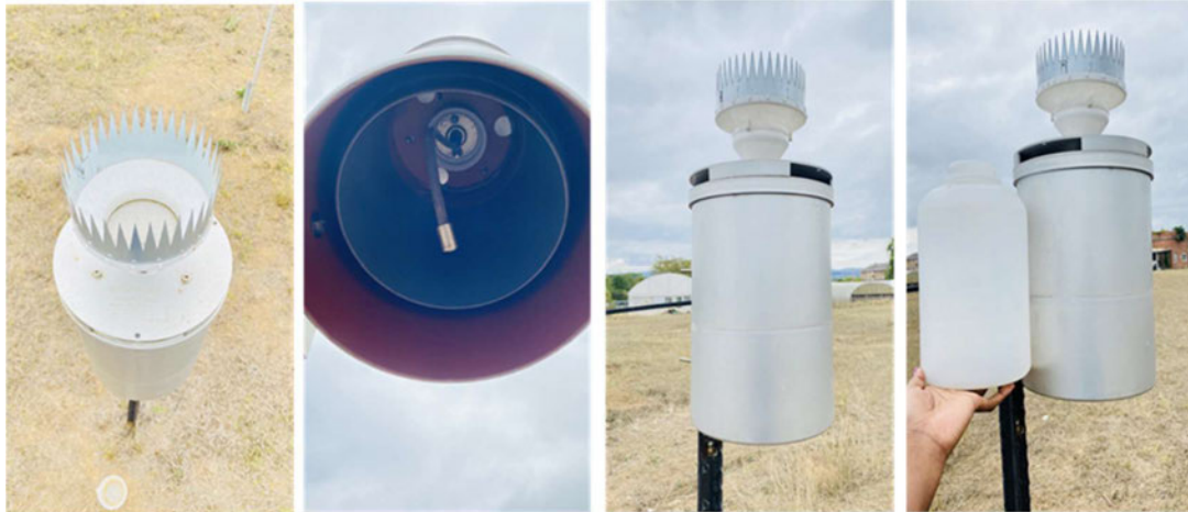
Figure 3.10 Side view of the rainfall station, showing funnel attached to metal protector, plastic siphon tube and plastic bottle.
