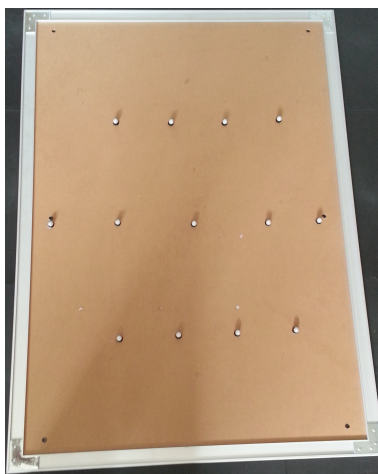
Figure 3.16: Calibration board that consist of reflective markers
