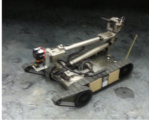
Figure 4.2: iRobot 510 PackBot with the ToF-IMU system mounted rigidly on the manipulator
