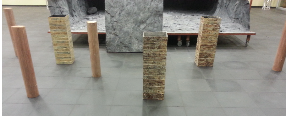
Figure 4.5: The environment where the robot moves in a 2D planar surface, with pillars to imitate the mining environment
