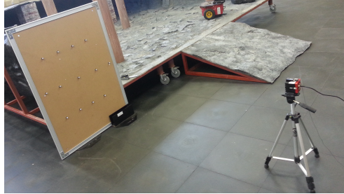
Figure 4.21: ToF-IMU system calibration setup showing ToF-IMU system on the tripod and the calibration board placed vertically
