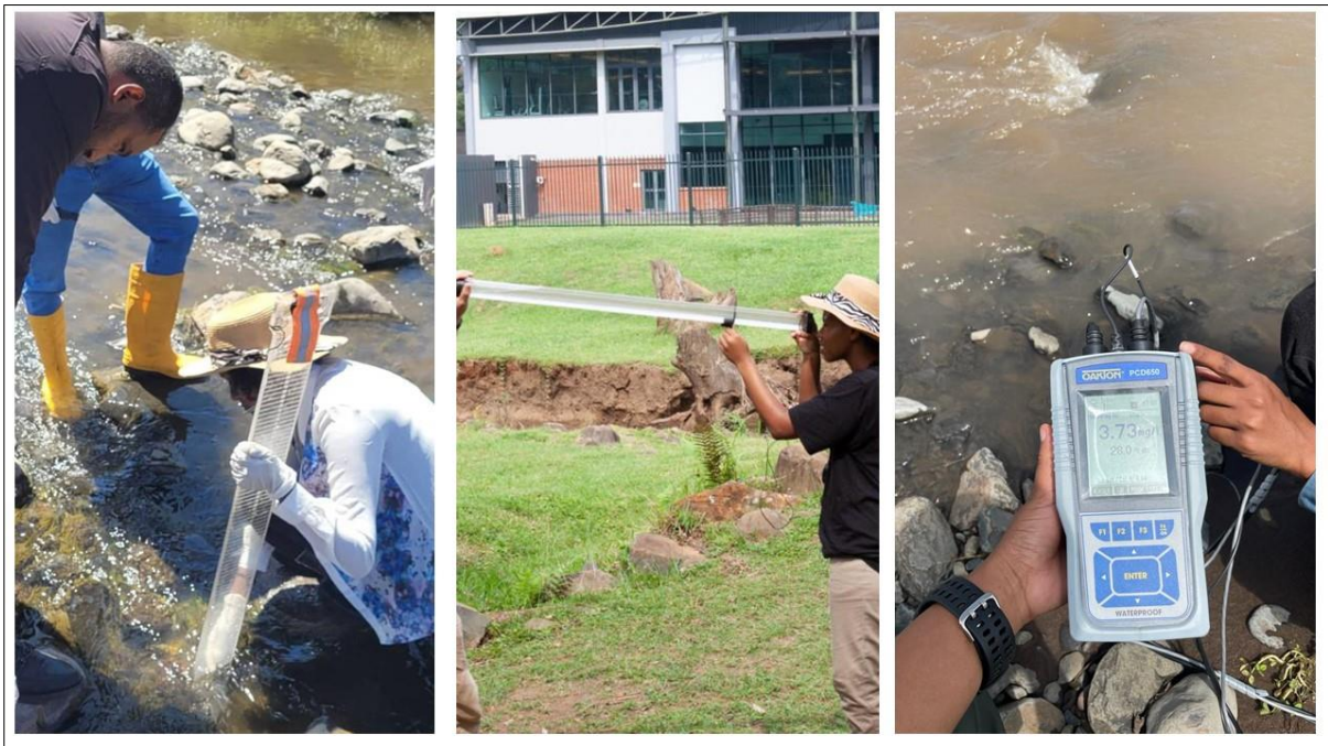
Figure 3.5 Transparent velocity head rod (left), Clarity tube (middle) and multiparameter PCD650 meter (right)
