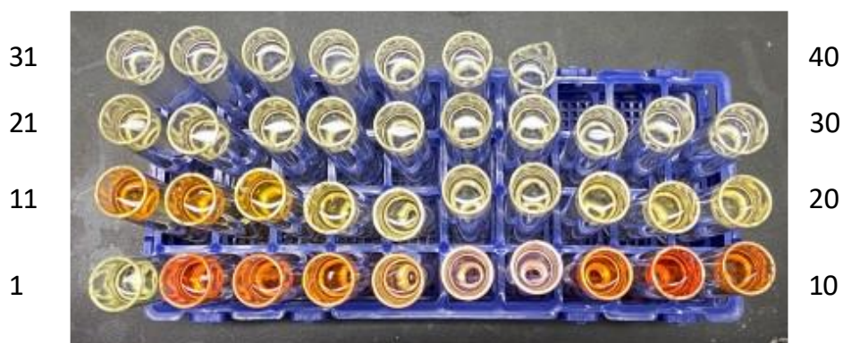
Figure 3.13: Different coloured fractions collected from silica gel chromatography.
