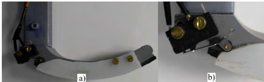
Figure 6-8: a) Heel strike detection micro switch, b) Close up view of the micro switch
