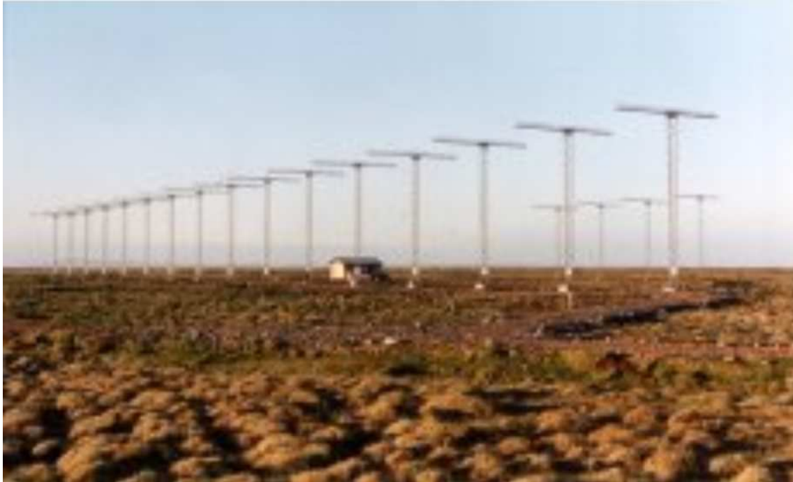
Figure 2.10: The primary array 16 log-periodic antennae and the secondary array of 4 antennae in the background (adapted from http://superdarn.jhuapl.edu ).
