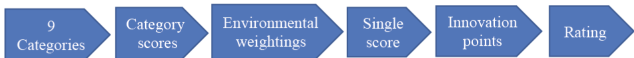
Figure 2.6: Procession of assessment credits in the Green Star SA Office technical manual v1.1. (Green Star SA, 2014)
