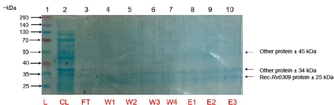
Figure 3.44: SDS-PAGE gel showing purification of recombinant Rv0309 in pET28a vector using Kumar et al. , 2013 protocol as guide. Samples were analysed using an 15% reducing Tris-glycine SDS-PAGE gel stained with Coomassie blue. Lane 1: Thermo Scientific Spectra Multicolour Broad Range Protein Ladder (L), Lane 2: Clear lysate (CL), Lane 3: Flow-through (FT), Lane 4: Wash 1 (W1), Lane 5: Wash 2 (W2), Lane 6: Wash 3 (W3), Lane 7: Wash 4 (W4), Lane 8: Eluent 1 (E1), Lane 9: Eluent 2 (E2), Lane 10: Eluent 3 (E3).
