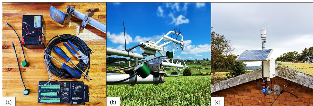
Figure 3.4 (a) The NDVI sensor setup in the laboratory, (b) its installation at the study site, and (c) the AWS at the high school in Swayimane.
