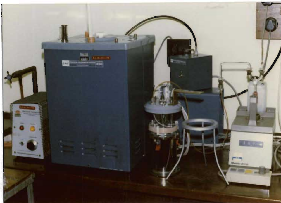
Plate 1 The titration calorimeter assembly. From left to right: the proportional controller, thermostatic bath, calorimeter unit, stirrer driver unit and automatic burette.
