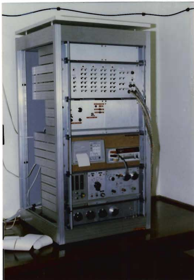
Plate 2 The titration calorimeter electronic assembly.
