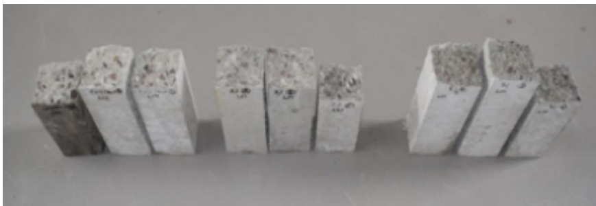
FIGURE 22. FAILURE ANALYSIS SAMPLE SOURCE - FLEXURAL STRENGTH BEAM FAILURE SURFACE ( SMITH 2019 )
