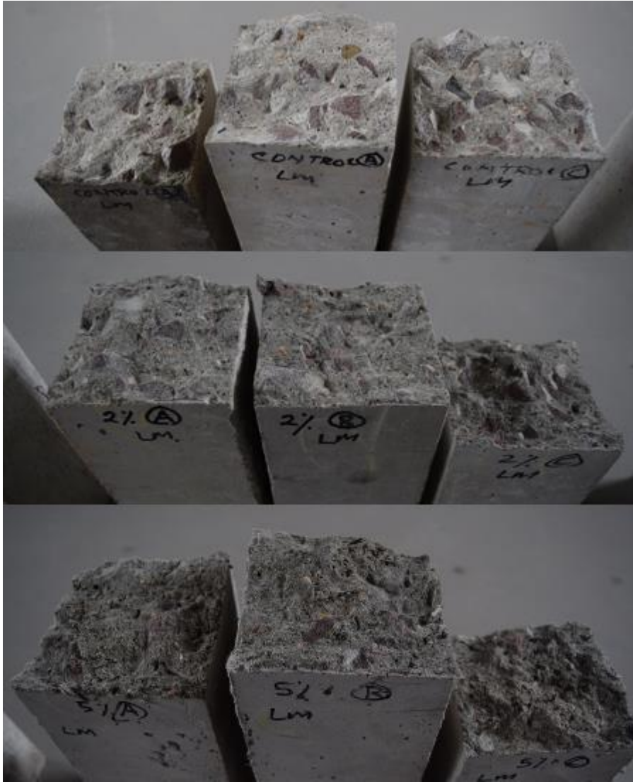
FIGURE 51. FAILURE ANALYSIS SAMPLE SOURCE - FLEXURAL STRENGTH BEAM FAILURE SURFACE - CLOSE UP (SMITH 2019)
