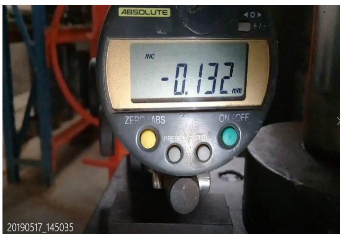
FIGURE 21. FOUR POINT BENDING - DISPLACEMENT MEASUREMENT ( SMITH 2019 )
