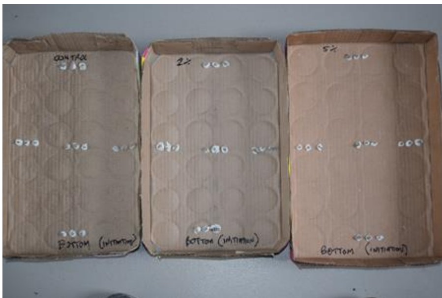
FIGURE 24. MICROSCOPY TEST SAMPLES REMOVED FROM FLEXURAL TEST BEAMS (SMITH 2019)
