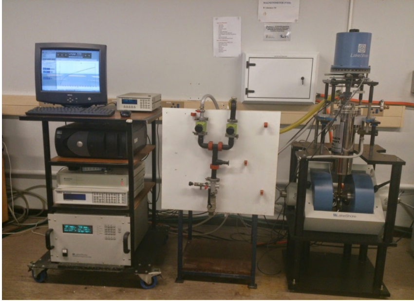
Figure 5.8: Lakeshore 735 Vibrating Sample magnetometer, Condensed Matter Physics Laboratory (WC), UKZN.
