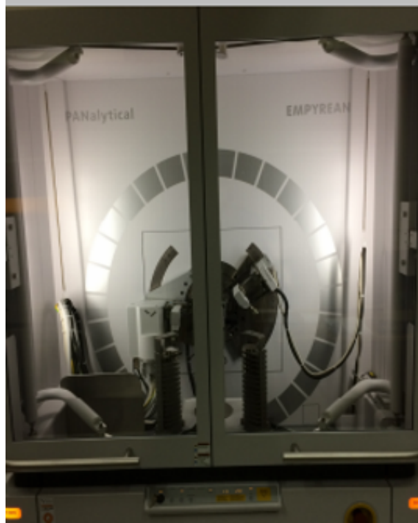
Figure 5.5: PW 1710 Empyrean PANalytical X-ray diffractometer, Geology (WC), UKZN.
