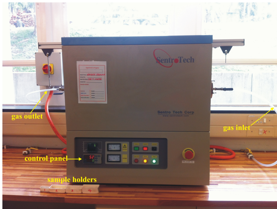
Figure 5.16: Sentro Tech high temperature furnace (type: STT-1600C-3-24).
