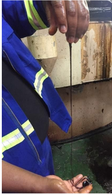
Figure 2.6: Rope-like Hard-to-boil sample tested using string proof test done by Noodsberg factory workers
