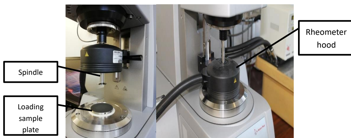
Figure 3.20: Spindle of Rheometer in loading position (L) and loaded position with hood (R)
