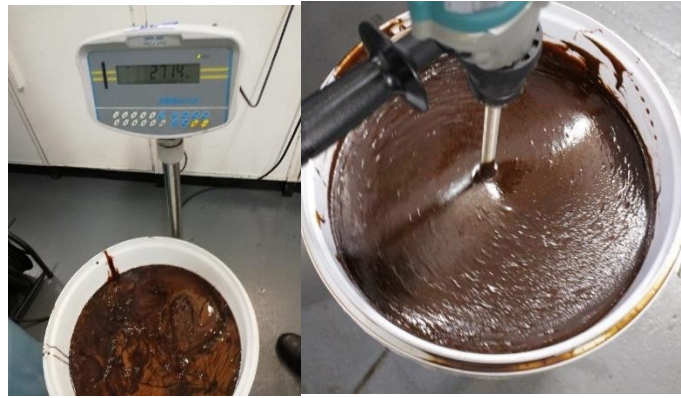
Figure 4.5: Dilution technique for massecuite samples: weighing samples (L) stirring samples (R)
