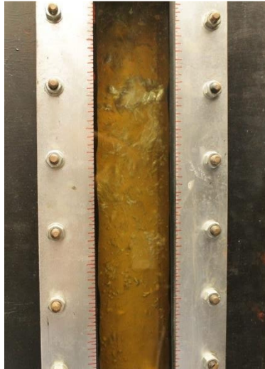
Figure 3.6: Boiling in Vacuum Pan Rig
