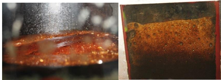
Figure 5.9: Foaming due to good (L) and HTB (R) samples
