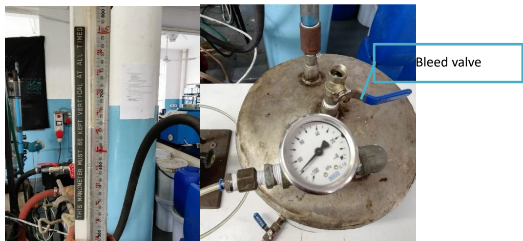
Figure 3.10: Pressure gauge test setup with manometer
