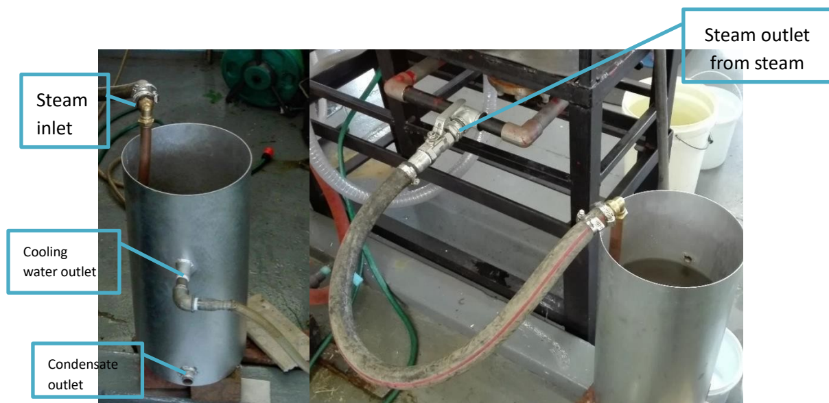
Figure 3.9: Steam side condenser
