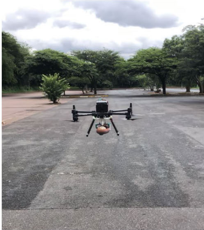
Figure 8-9: ISP-UAV Assembly Hovering During Final Flight Test
