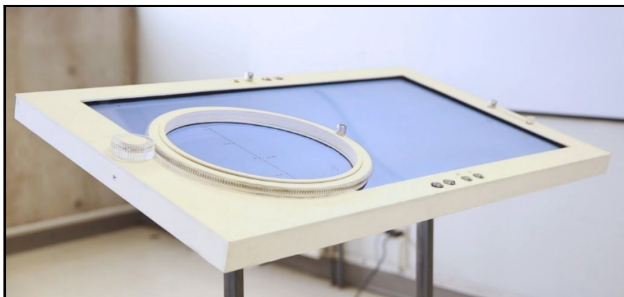
Tangible mathematics interface designed to learn trigonometry.
