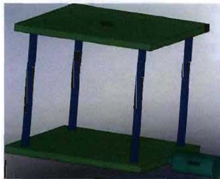
Figure 4-6 Quadruple vertical lead-screw design.
