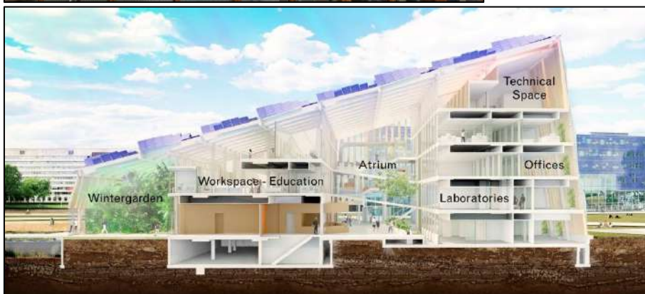
Figure 5.6: The Diagram on the left shows The Energy Academy Europe sectional Elevation of internal spaces
