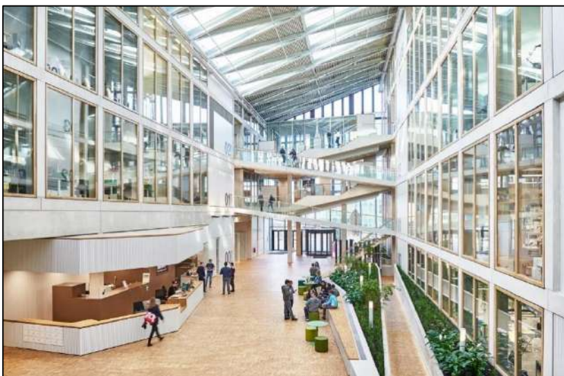
Figure 5.2: The Picture shows the natural lighting that is provided by the Atrium to the internal workspaces through large glass windows. This visibility and large open pause spaces allow for social interaction and improve productivity to take place.
