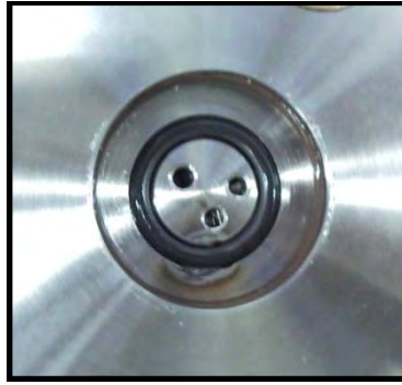
Photograph 4-2: The O-rings in the upper 316 stainless steel flange that seal the equilibrium cell.
