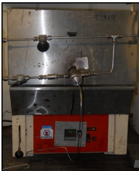
Figure 3-4: The oven with the temperature controller and thermocouple
