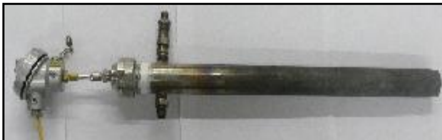
Figure 3-5: Fixed Bed Reactor
