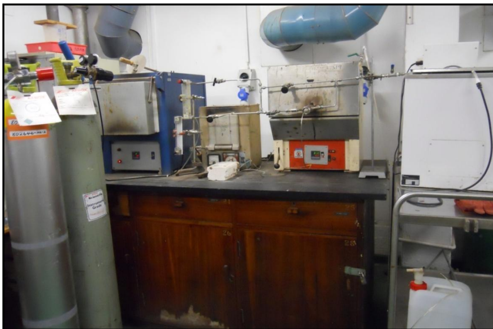
Figure 3-1 : The Testing unit developed for Desulphurization of flue gas
