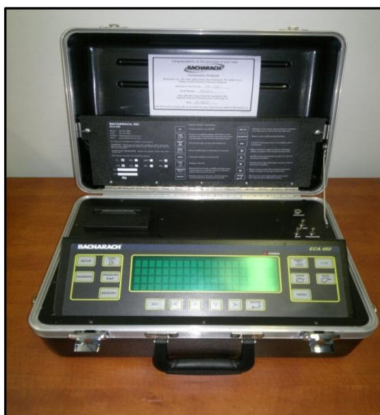
Figure 3-8: Portable Gas Analyzer
