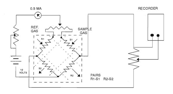
FIGURE 4.7. CIRCUIT DIAGRAM OF GOW-MAC T.C.D. DETECTOR
