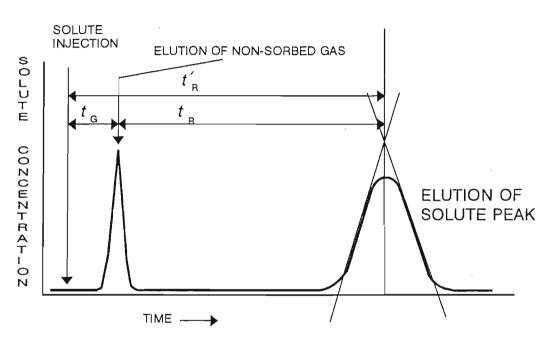
FIGURE 4.8. A Typical Chromatogram Showing the Determination of the Retention Time of a Solute Using the Tangents to The Peak Method
