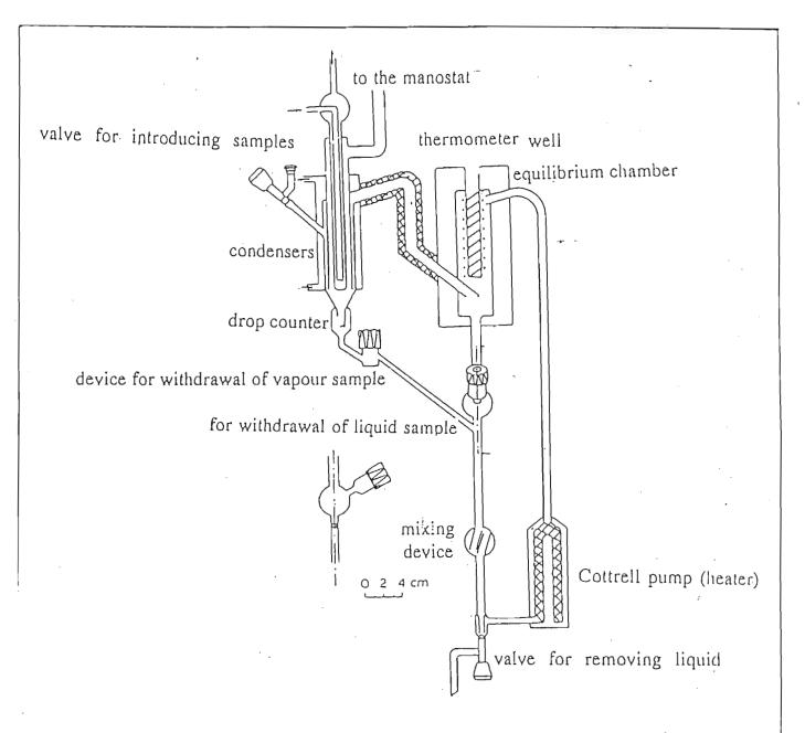
The Ebulliometer allowing the withdrawal of the Samples in Equilibrium
