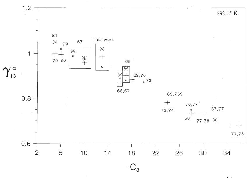
FIGURE 4.9. Diagram of Carbon Number of the Solvent (C<sub>3</sub>) where, represents pentane, + represents hexane and \* represents heptane
