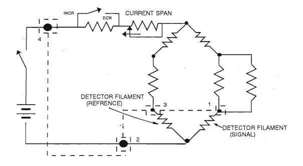
FIGURE 4.6. CIRCUIT DIAGRAM OF THE SHANNDON UK3 T.C.D. DETECTOR
