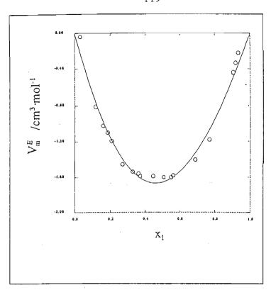
FIGURE 5.5. Excess Molar Volumes of 1-Heptyne versus Sulfolane at 303.15 K FIGURE 5.6. Partial Molar Volumes of 1-Heptyne and Sulfolane at 303.15 K
