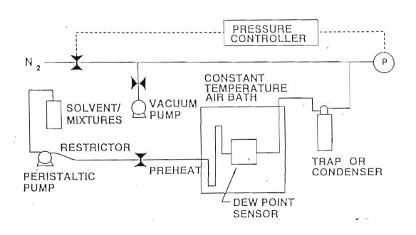
FIGURE 2.8. Overall design of the system used to measure the Activity coefficient at infinite dilution by dew point measurements. (32)
