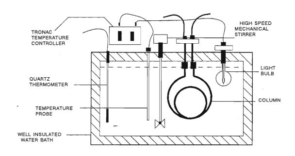
FIGURE 4.3. WATER BATH FOR TEMPERATURE CONTROL AT 298.15 K
