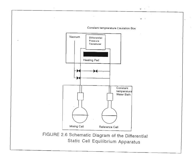
Once the solvents have been boiled, the cells are placed in an ultrasonic bath for further degassing. A vacuum is again applied to one cell at a time for approximately 3-5 minutes, and the cycle is repeated 4-6 times. If the solvent is moderately volatile, the procedure is similar except that degassing cycles are shorter. Alternatively, freeze-thaw cycles using liquid nitrogen are used for very volatile solvents.
