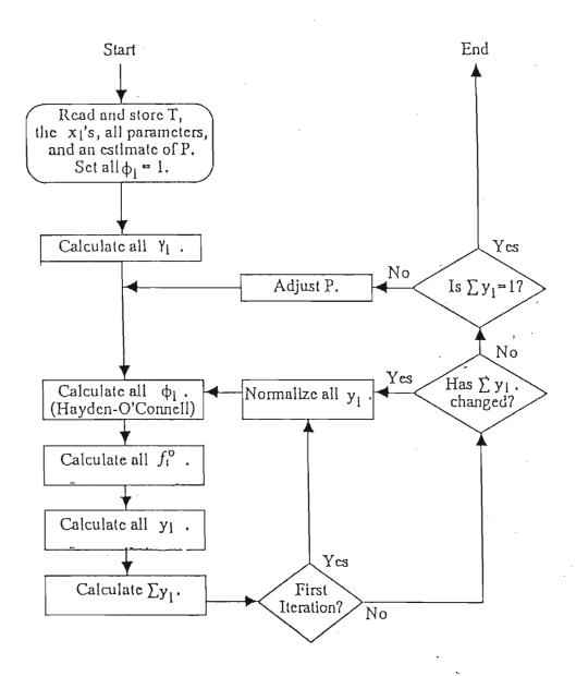
FIGURE 7.4. An Algorithm for the Simultaneous Solution for P and y<sub>i</sub>
