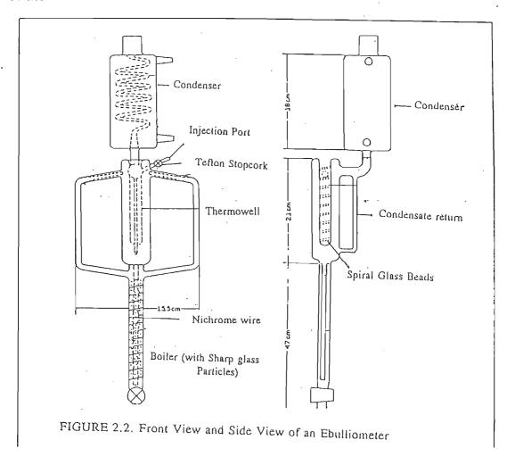
liquid is taken up by evaporation. The remaining liquid passes down the outsides of the thermowell, slowed by helical beads, returns via the inner cylinder, and is joined by the cooled condensate. The whole ebulliometer is thoroughly insulated.
