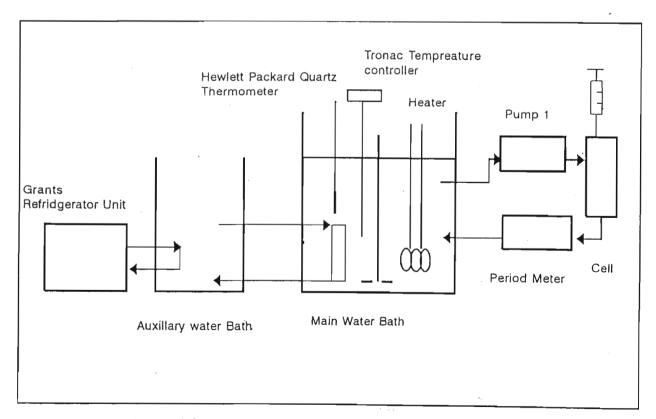
Figure 5.2 Laboratory arrangement for the glc apparatus
