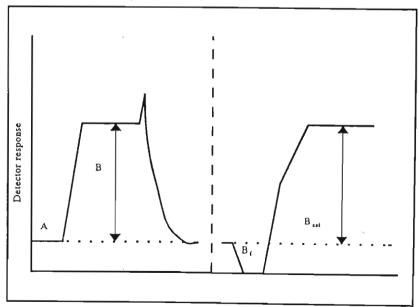
FIGURE 6.2. A typical Calibration and Experimental recorder output for the LKB microcalorimeter
