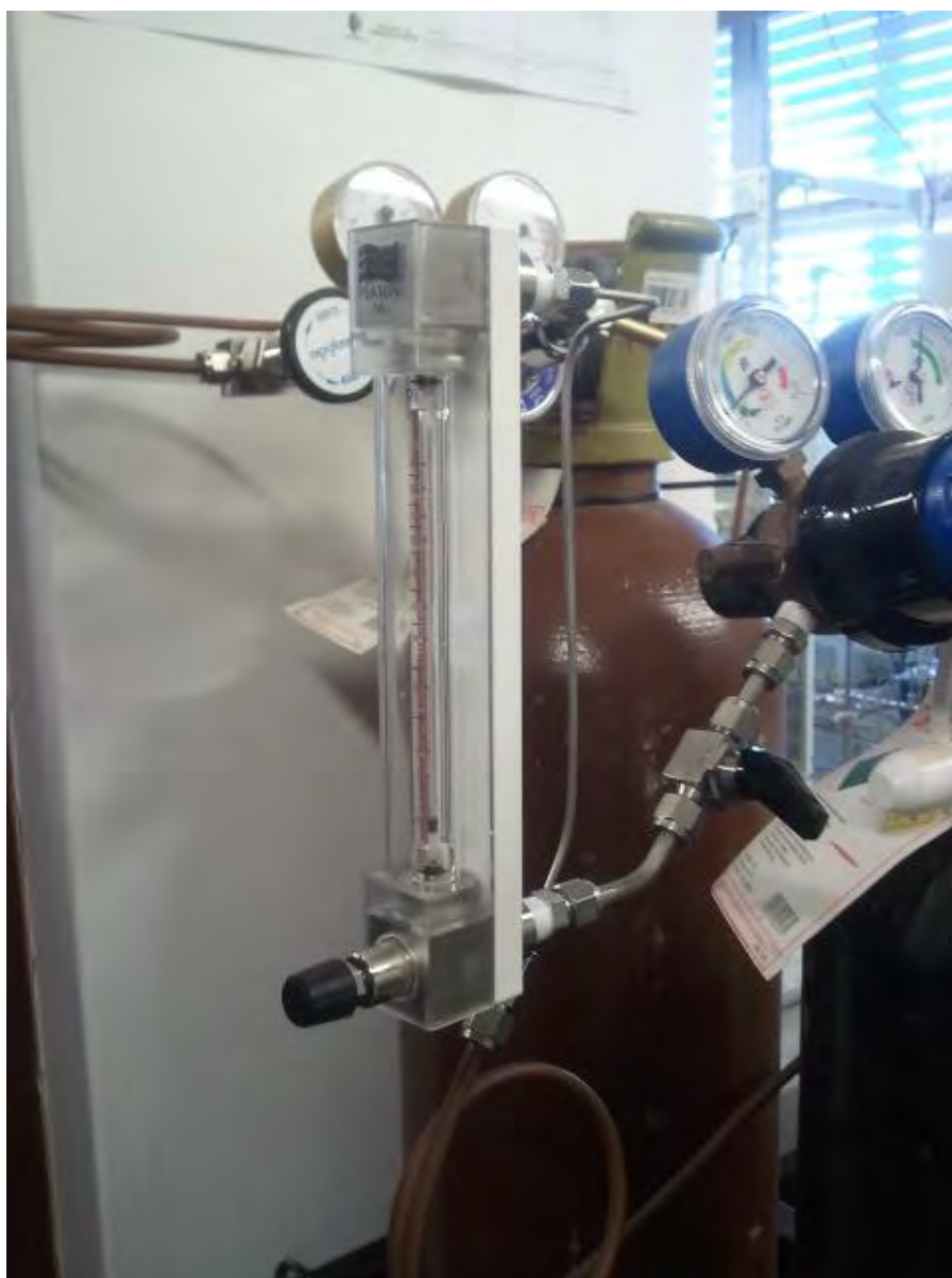
Photograph 3.11. Platon quartz glass rotameter for low feed-gas flow-rates.
