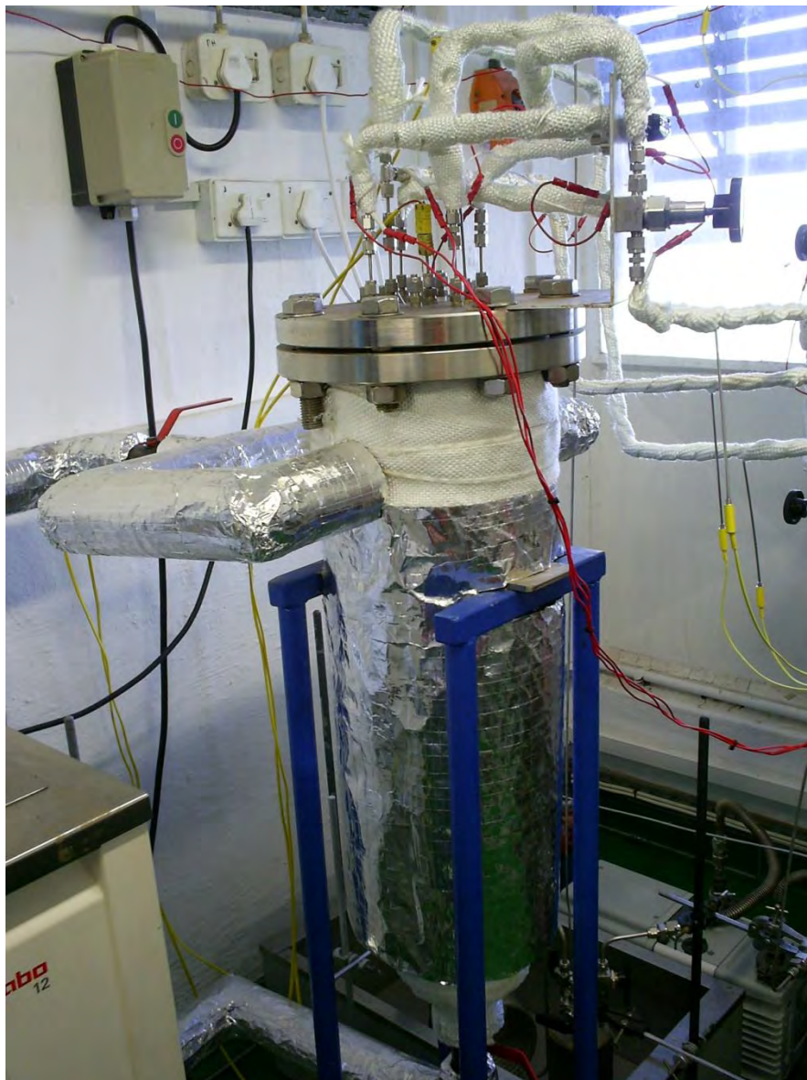
Photograph 3.3. Fully commissioned laminar flow HFP oxidation reactor.
