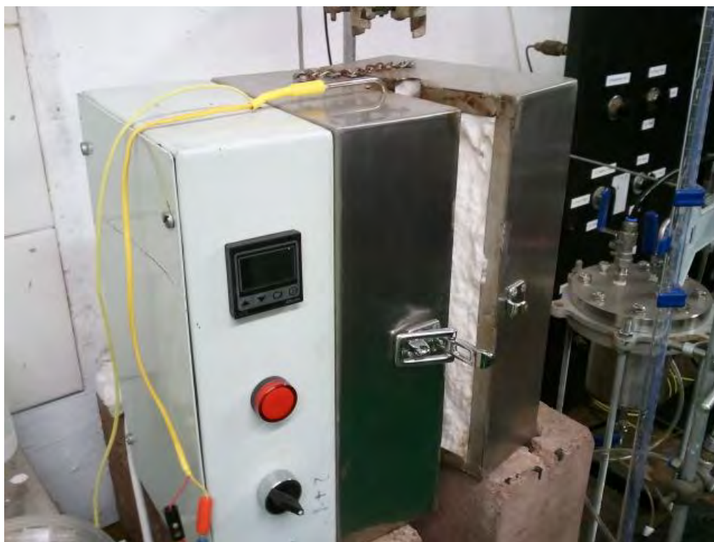
Photograph 3.15. Tube furnace used for the calcination of the copper-based, silica-supported HFP oxidation catalysts.
