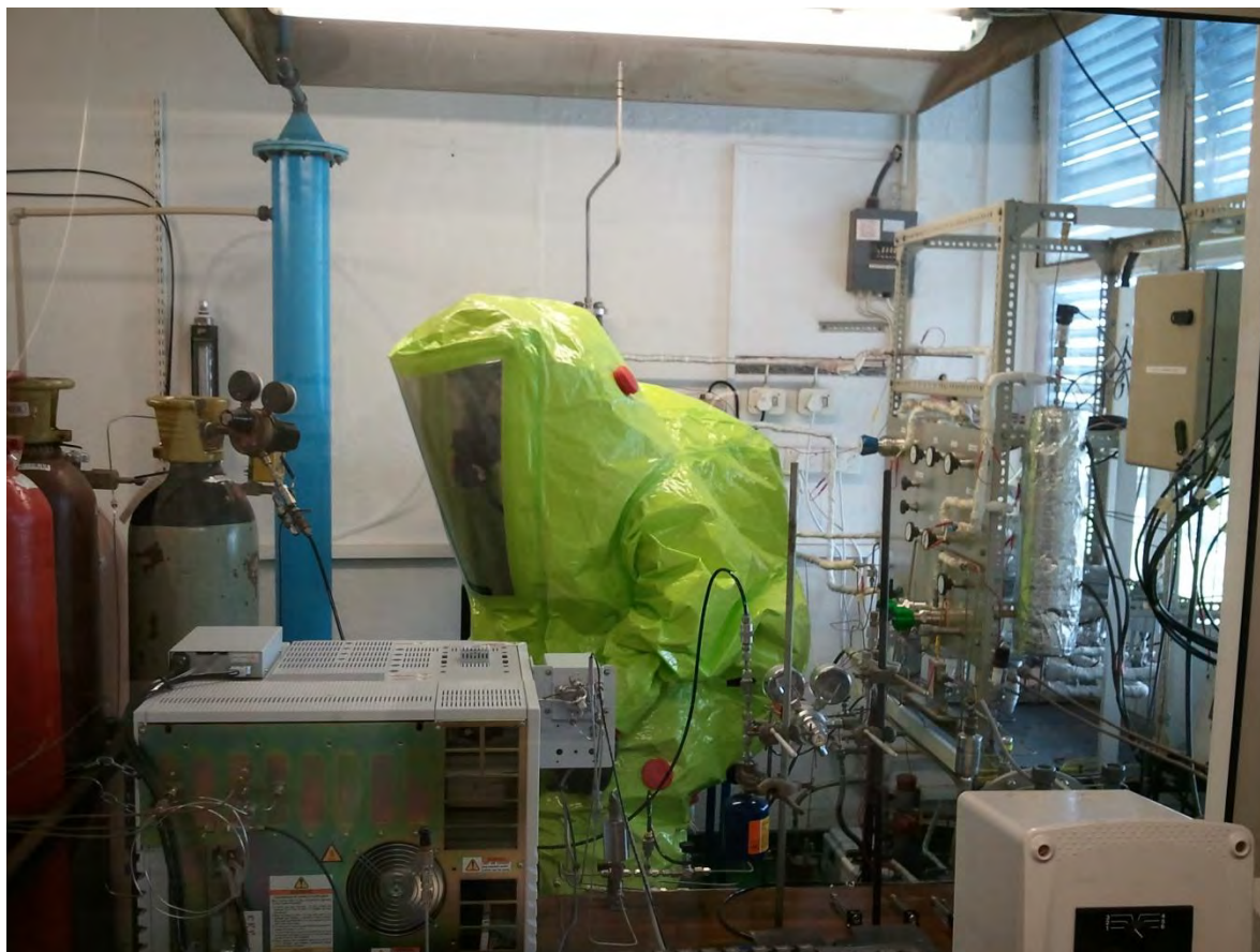
Photograph 3.17. Gas-chromatograph detector calibration for a toxic gas, undertaken using a full-body hazardous materials suit and self-contained breathing apparatus.
