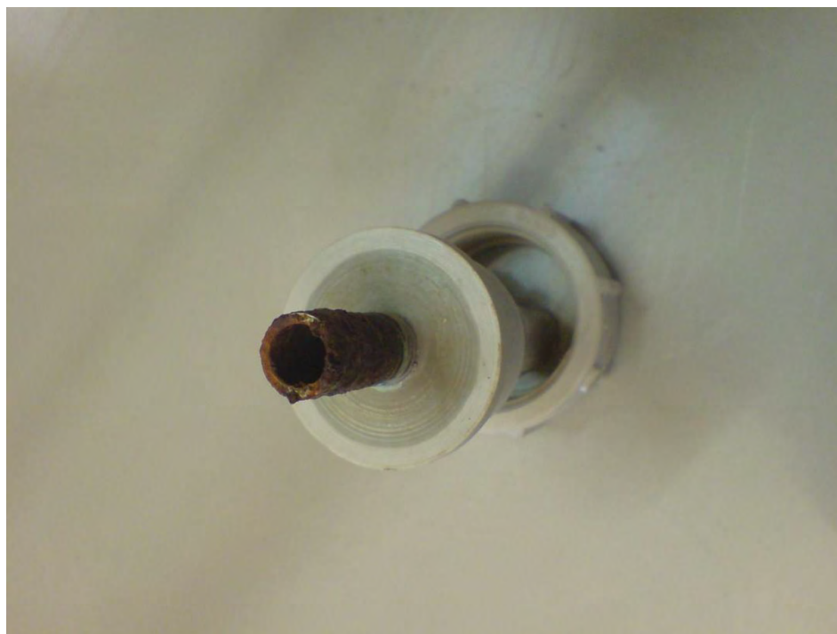
Photograph 3.8. Corrosion of stainless-steel tubing connected directly to the caustic scrubber unit.
