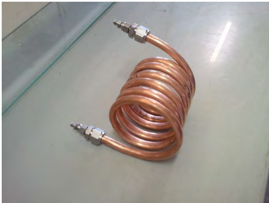
Photograph 3.12. Coil-type fixed-bed reactor used for the study of the catalytic oxidation of HFP.
