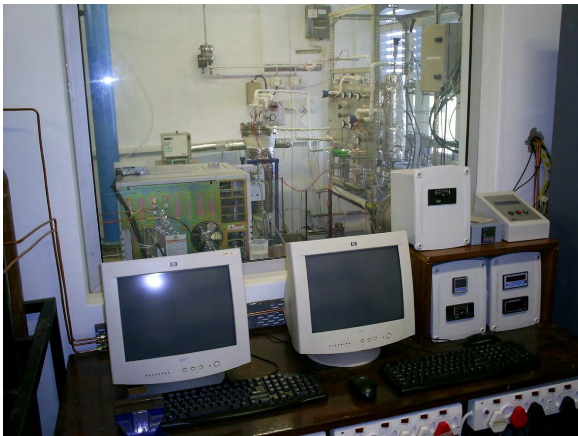
Photograph 3.6. View of the non-catalytic HFP oxidation apparatus, from the control room.
