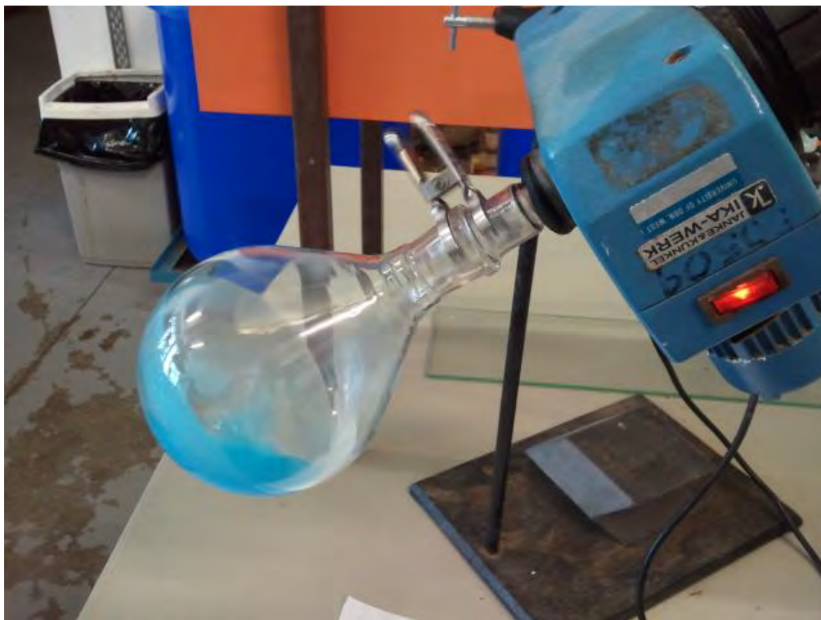
Photograph 3.14. Silica gel and copper nitrate trihydrate agitated and aged for 18 hours.
