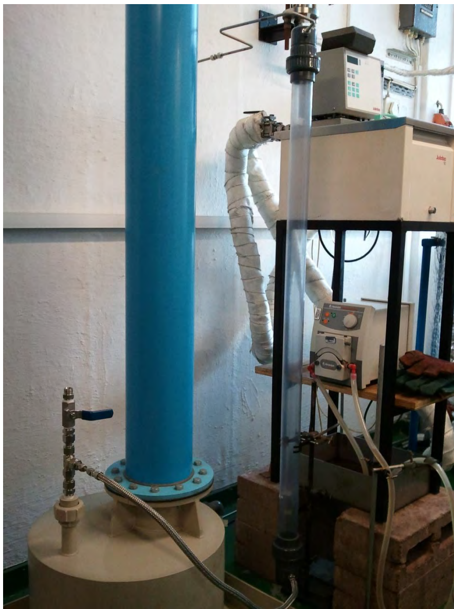
Photograph 3.9. Installation of a transparent, polypropylene guard column at the inlet of the caustic scrubber unit.
