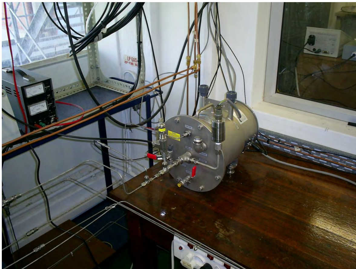
Photograph 3.4. Ritter drum-type wet-test meter (model TG05) used for the measurement of feed and product-gas volumetric flow-rates.
