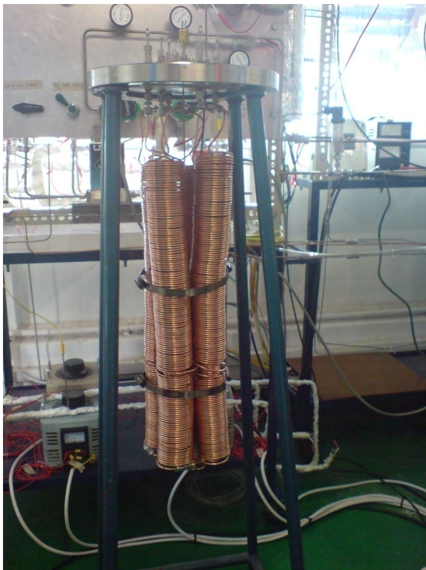
Photograph 3.2. Copper reactor coils fixed to the top blind-flange of the stainless steel heating jacket.
