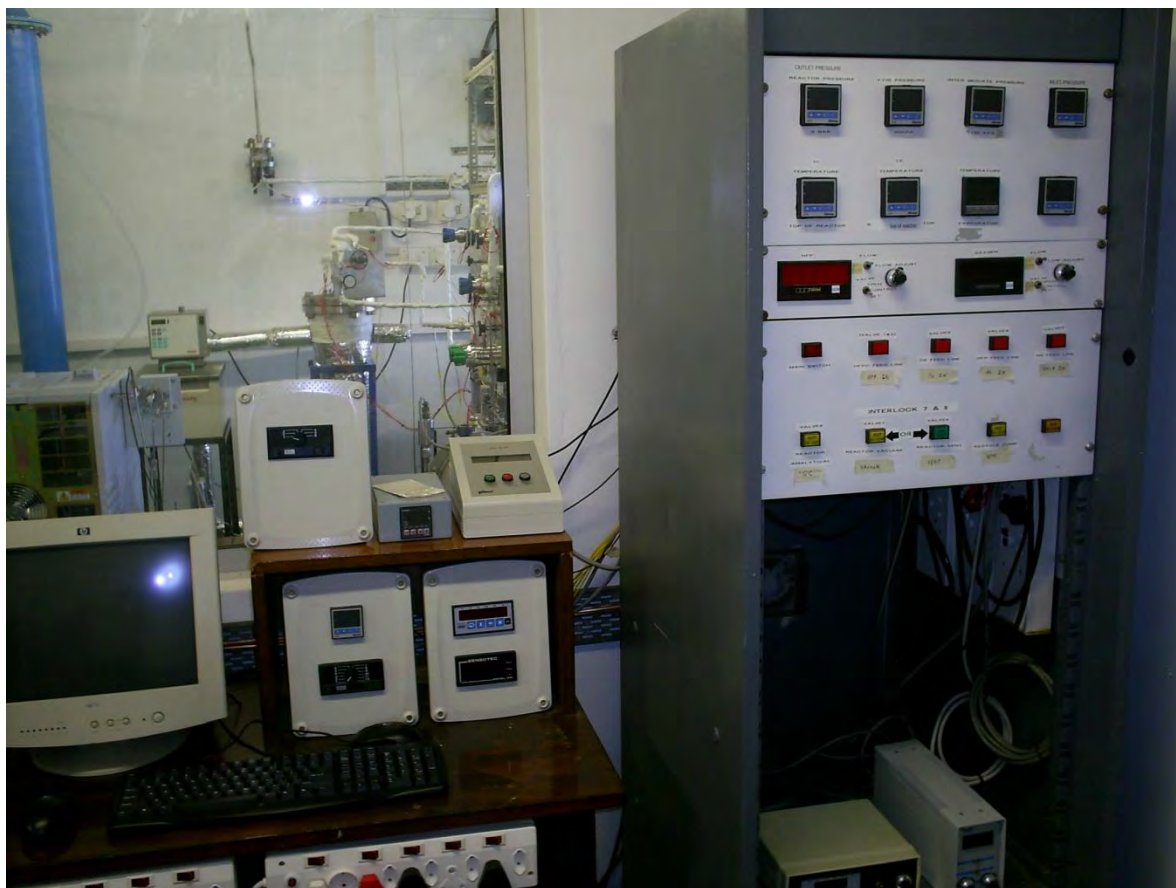
Photograph 3.7. HFP oxidation apparatus display and control units.
