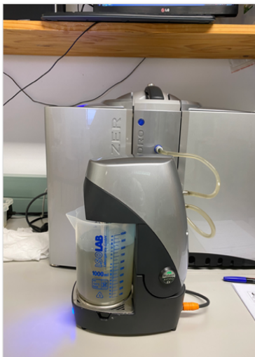
Figure 25: Malvern Mastersizer 3000 used to determine particle size distribution.
