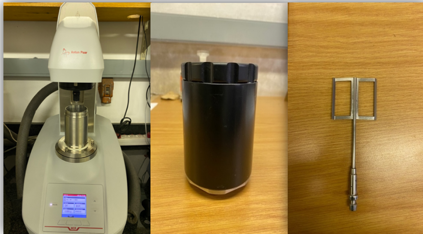
Figure 26: Rheometer and vane in cup geometry used to determine shear stress.
