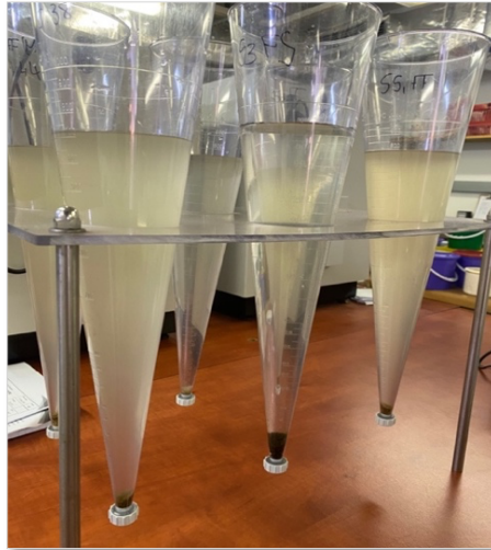
Figure 27: Settled sludge volume in Imhoff cones during the SVI tests.
