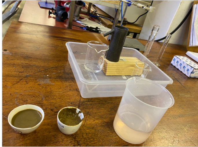
Figure 23: Experimental setup used to measure the density of faecal material.
