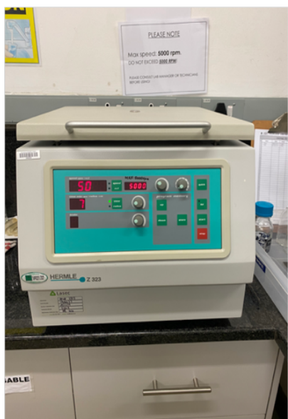
Figure 22: Centrifuge used to separate the liquid phase from the solid phase.
