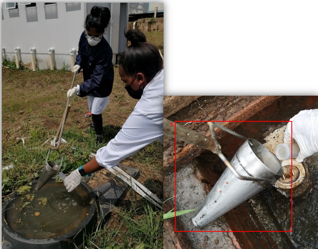
Figure 16: Image of sampling tool and method for collection of faecal material.
