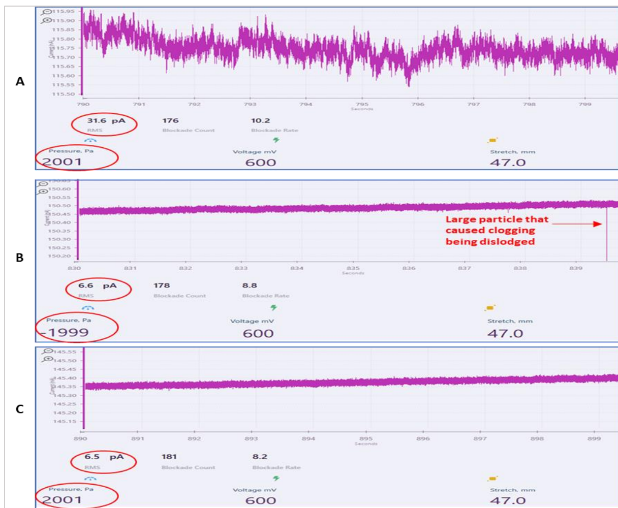
Figure 3.3: Unclogging a nanopore. A) Typical profile indicating a clogged nanopore identifiable by unstable baseline current and elevated RMS noise of 31.6 pA. B) Unclogging the nanopore following the application of negative pressure of -1999 Pa causes a large particle to be dislodged and the baseline current stabilises, followed by a decrease in RMS noise to 6.6 pA. C) Once positive pressure reapplied at 2001 Pa, baseline current remains stable with the RMS noise remaining low at 6.5 pA.
