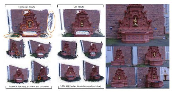
**Figure 11:** Our results of the Fountain reconstruction compared to Furukawa's models. The models are meshed and texture mapped from the respective patch models. The number of vertices of the patch models is indicated in the bottom of the image. It can be seen that with our method, we generate more patches than the baseline method. When we look at the Furukawa's results, we can notice some missing vertices which imply that our mesh models are more complete.
