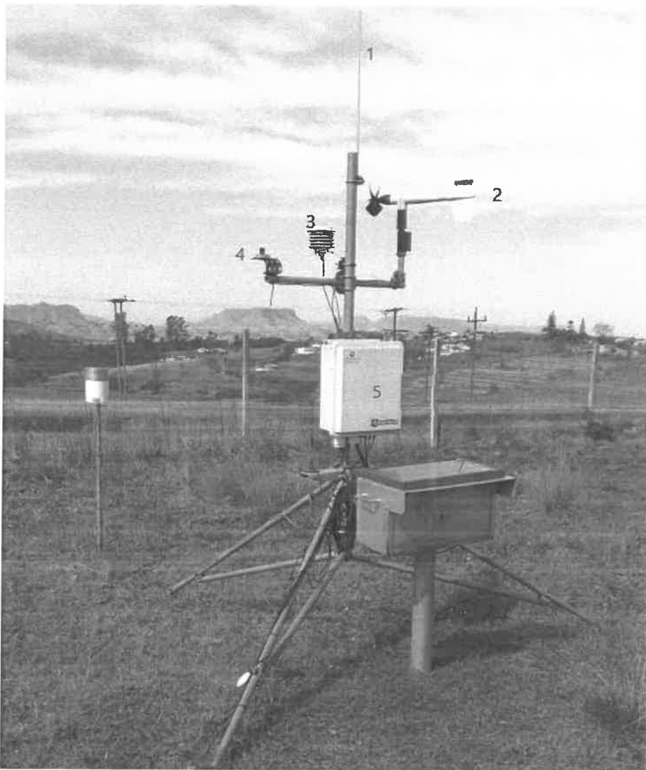
Figure 3.3: A picture of the AWS system installed at Swayimane High School with its different components
