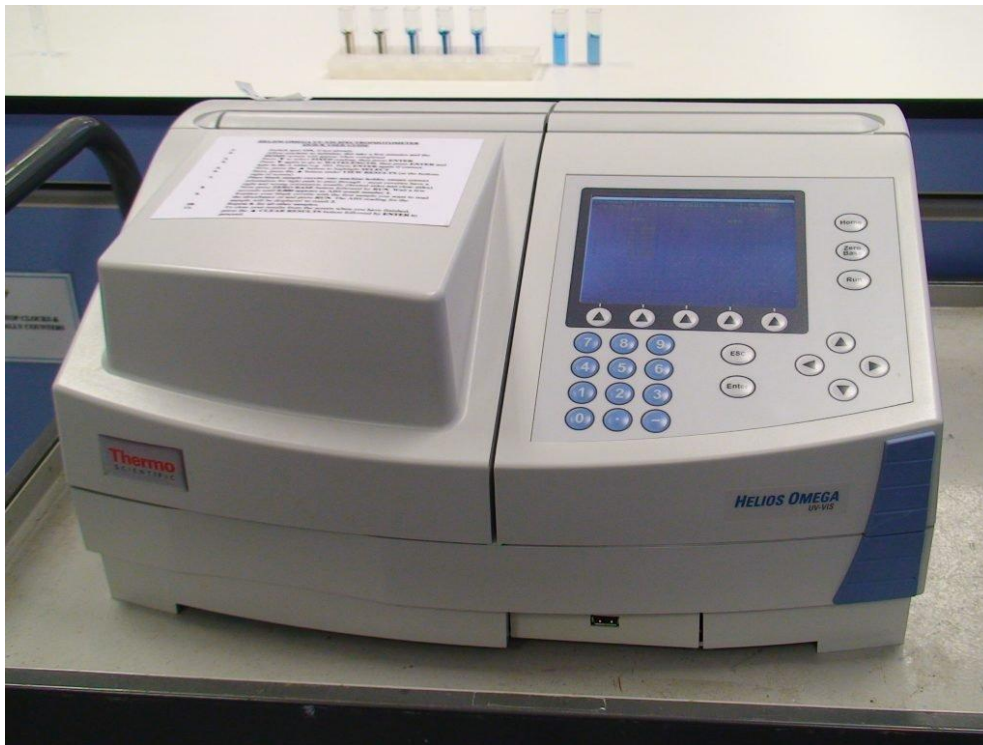
Figure 8.2: A typical spectrophotometer instrument seen in a lab (Source: Wikipedia Commons )
