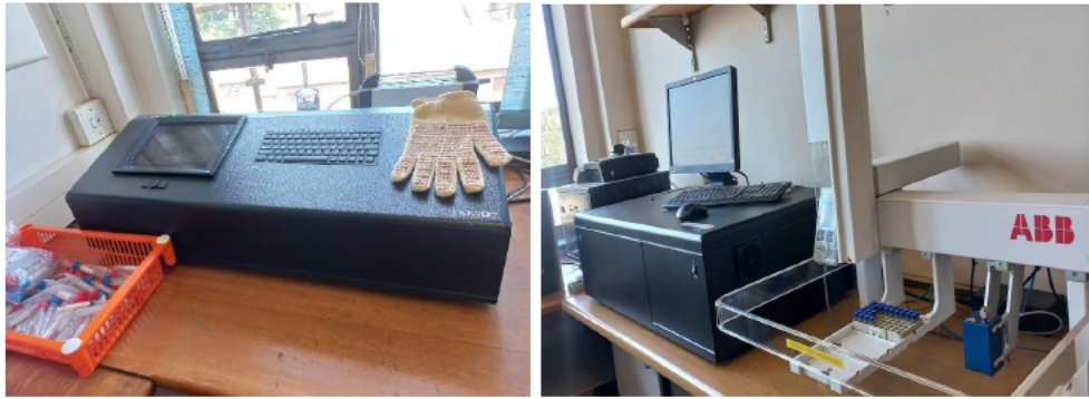
Figure 4.3: The Los Gatos Research (LGR) Liquid Water Isotope Analyser (LWIA) located at UKZN Agricultural Campus, Pietermaritzburg
