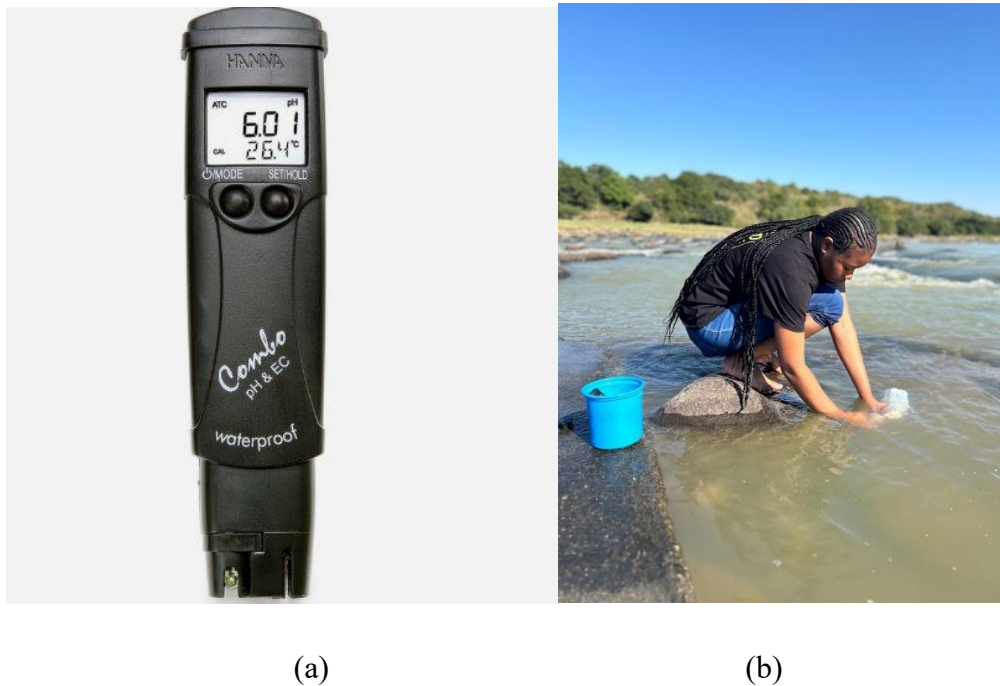
Figure 4.2: Portable multi-sensor meter (Hanna, 1996) (a) used to measure T, EC, and pH from water samples collected and pictures taken while sampling the Shu-Shu thermal springs (b)
