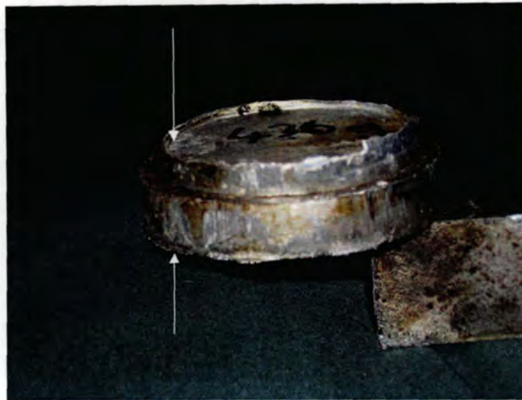
Diagram 4-30: Photograph showing Biscuit Thickness of Run #1
