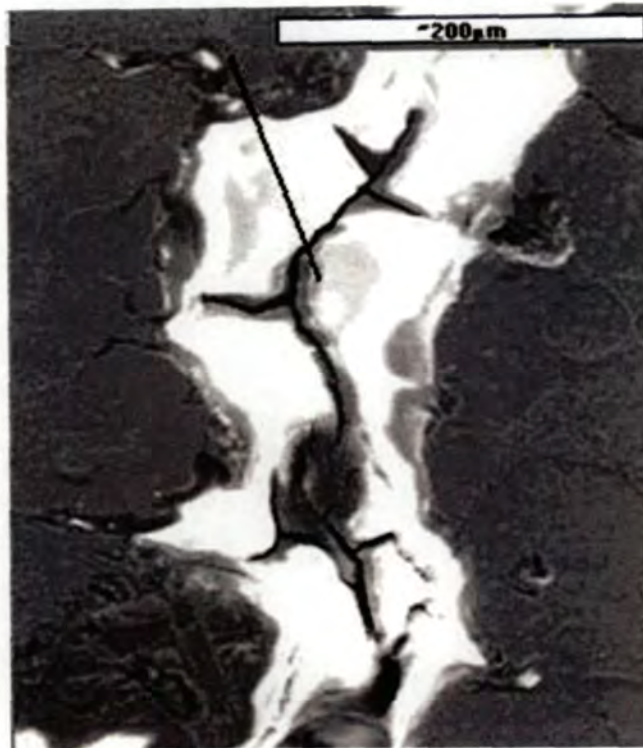
Diagram 4-13: SEM Microscopy of the Crack
