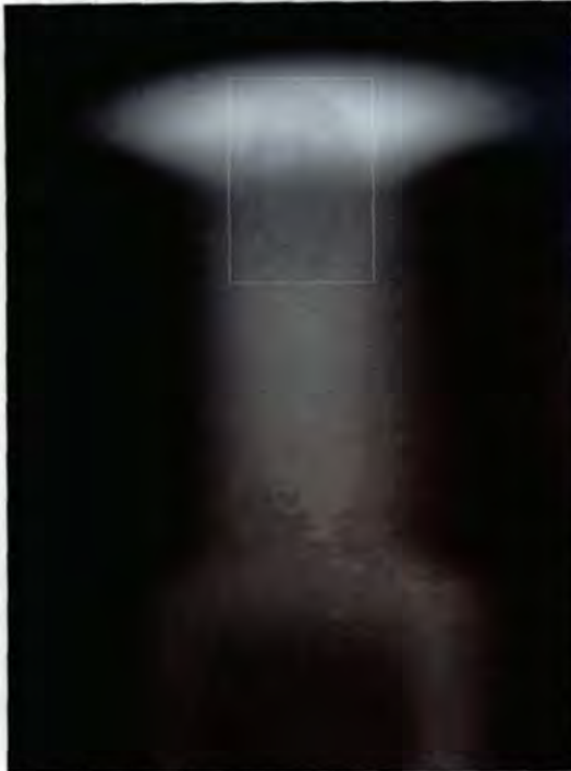
Diagram 4-15: Radiograph Showing Porosity
