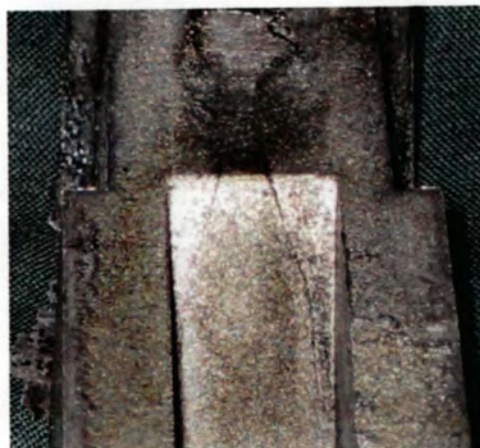
Diagram 4-28: Close up of Casting Run #3, Showing Crack
