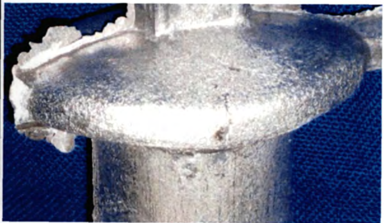
Diagram 4-57: Photograph of close up of section Component from Exp. 2 run 2 showing the defect shown in diagram 4-56
