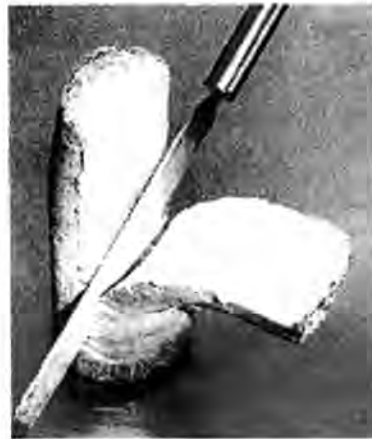
Diagram 2-11: Photograph illustrating SSM Behaviour [1]
