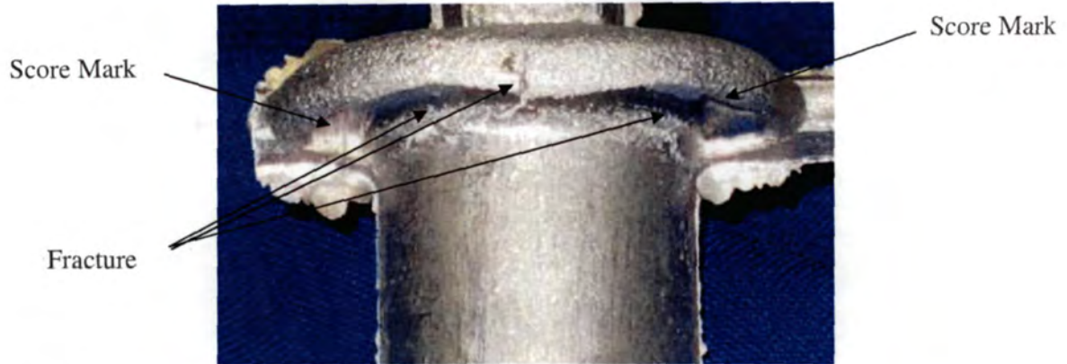
Diagram 4-58: Photograph of close up section of Component from Exp. 2 run 2 from underneath showing score marks
