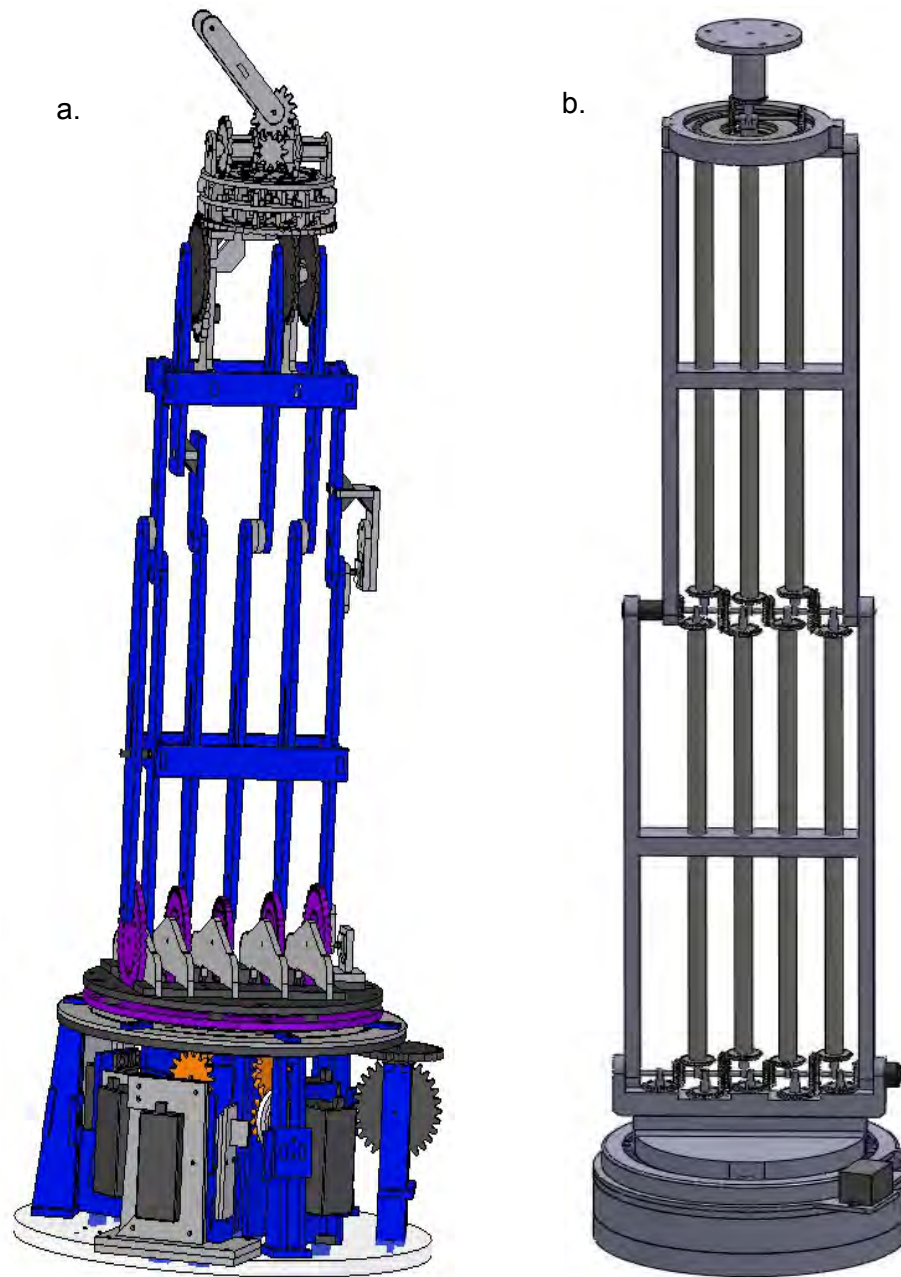
Figure 66: 6 DOF large workspace, low inertia machine designs
