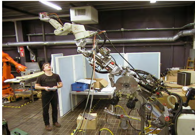
Figure 29: Hybrid reconfigurable manipulator from Sørensen, et. al. (2004) [69]
