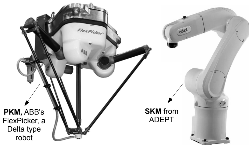
Figure 1: Comparative illustrations of a PKM and SKM
