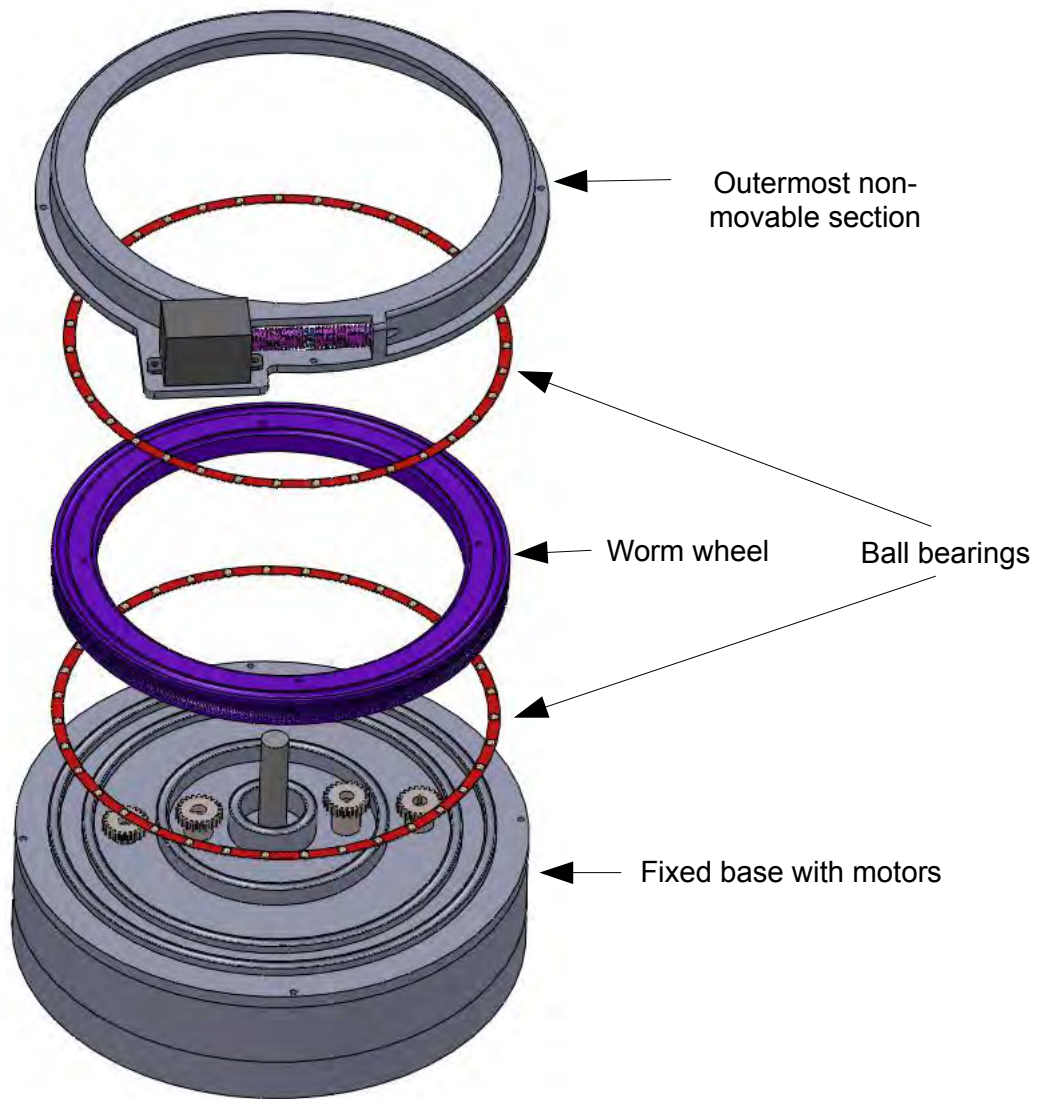
Figure 51: Outermost section securing 6 th movable section to fixed base
