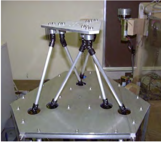
Figure 7: 6-PSU platform from Hopkins and Williams (2002) [54]
