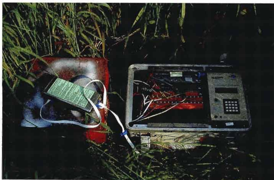
Fig. 4.6 The CR7X datalogger (right) and metal enclosure (left) for the batteries. On top of the enclosure is the datalogger storage module (Photo MJ Savage)
