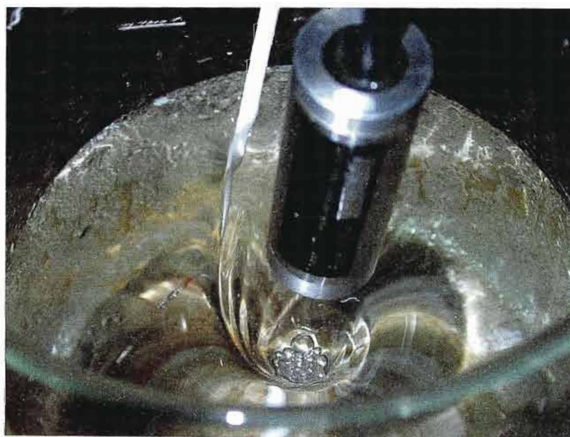
Fig. 5.1 A magnetic stirrer is used to create a whorl of water. The IRT measures the surface temperature of the water and a thermocouple the water temperature (Savage et al. , 2000)
