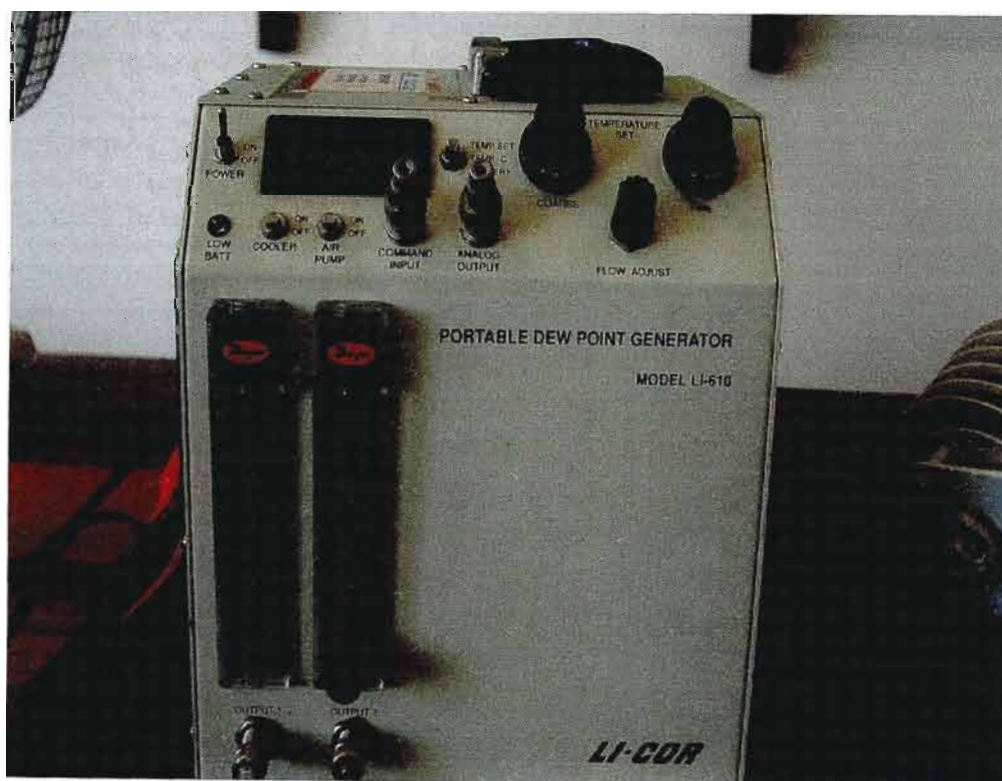
Fig. 5.2 The LI-610 portable dew point generator (Savage, 2002c)
