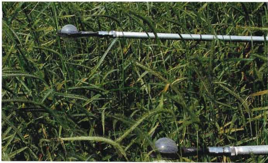
Fig. 4.3 Two net radiometers placed at 1.5 m above the soil surface facing north about 5 m apart from the weather station (Photo MJ Savage)
