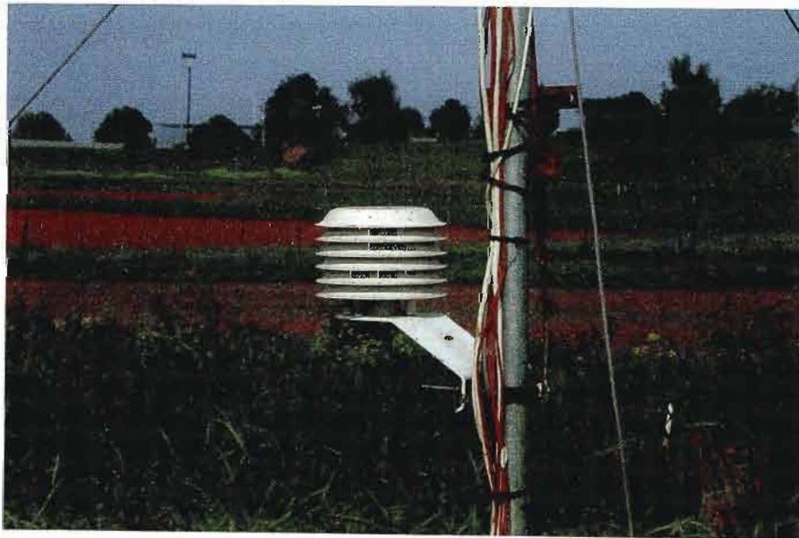
Fig. 4.2 Vaisala CS500 relative humidity and air temperature probe inside a 6-plate radiation shield (Photo MJ Savage)
