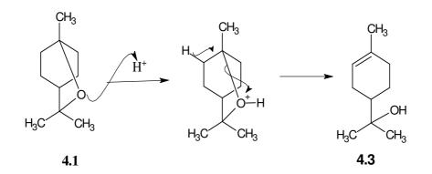
Scheme 4.1 Plausible mechanism for the conversion of 4.1 to 4.3
