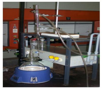
Figure 3.3 Clevenger apparatus for hydrodistillation of aromatic plants
