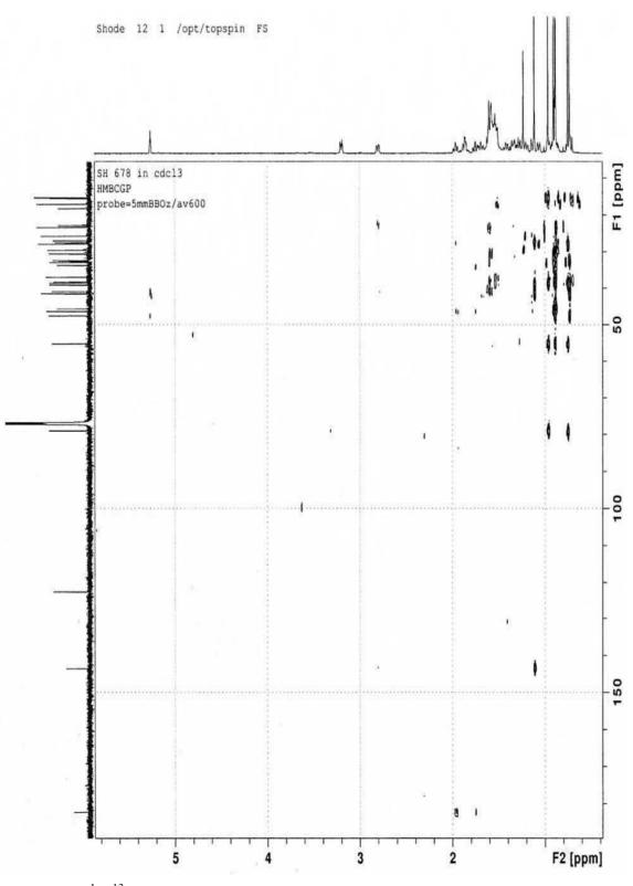
Figure 5.2.8: <sup>1</sup>H <sup>13</sup>C HMBC NMR Spectrum of **OO/55/A**
