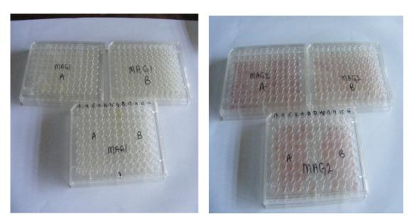
Figure 4.5: 96 Well plates (MIC) of the essential oils of *M. trichostachya* var. *compacta* (MAGI and MAG2)
