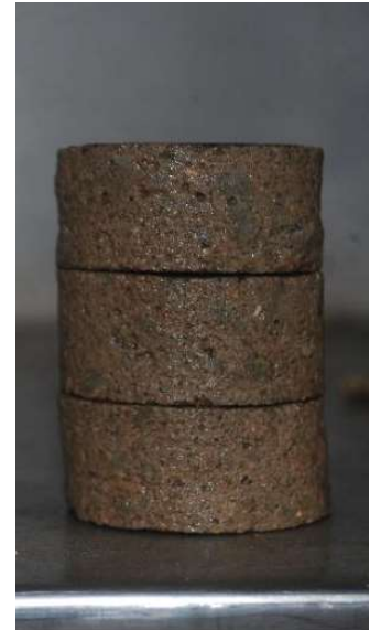
(b) Core samples after cutting
