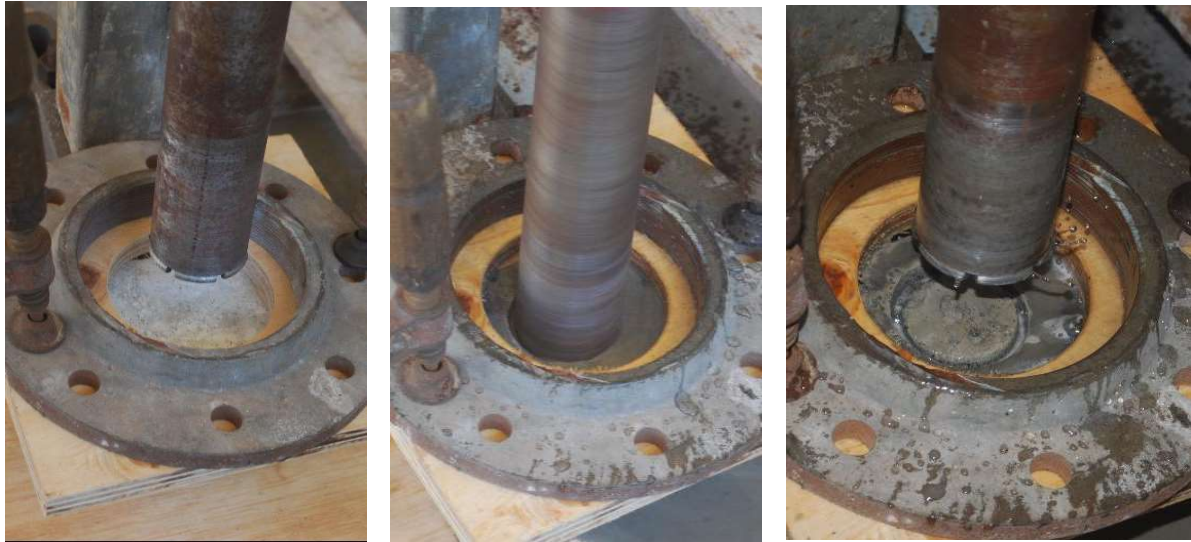
Figure 3-8: Coring of cube samples
