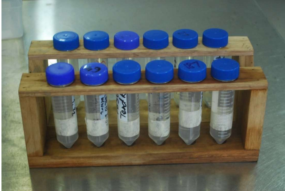
Figure 3-40: Wastewater samples prepped for ICP analysis
