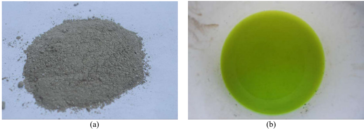
Figure 3-4: Penetron Admix (a) before the addition of water (b) after the addition of water
