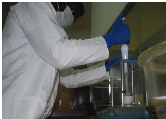
Figure 3-28: Measurement of wastewater sample into crucible
