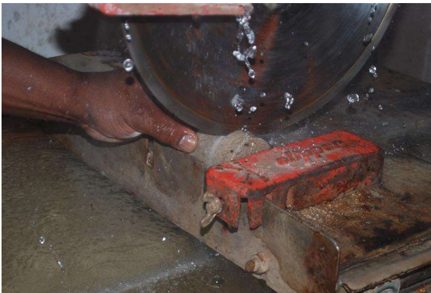
(a) Core samples during cutting
