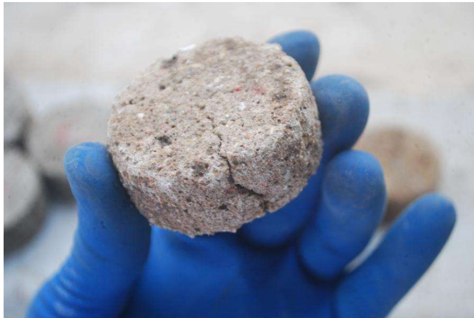
Figure 4-20: PC m sample after 9-month exposure
