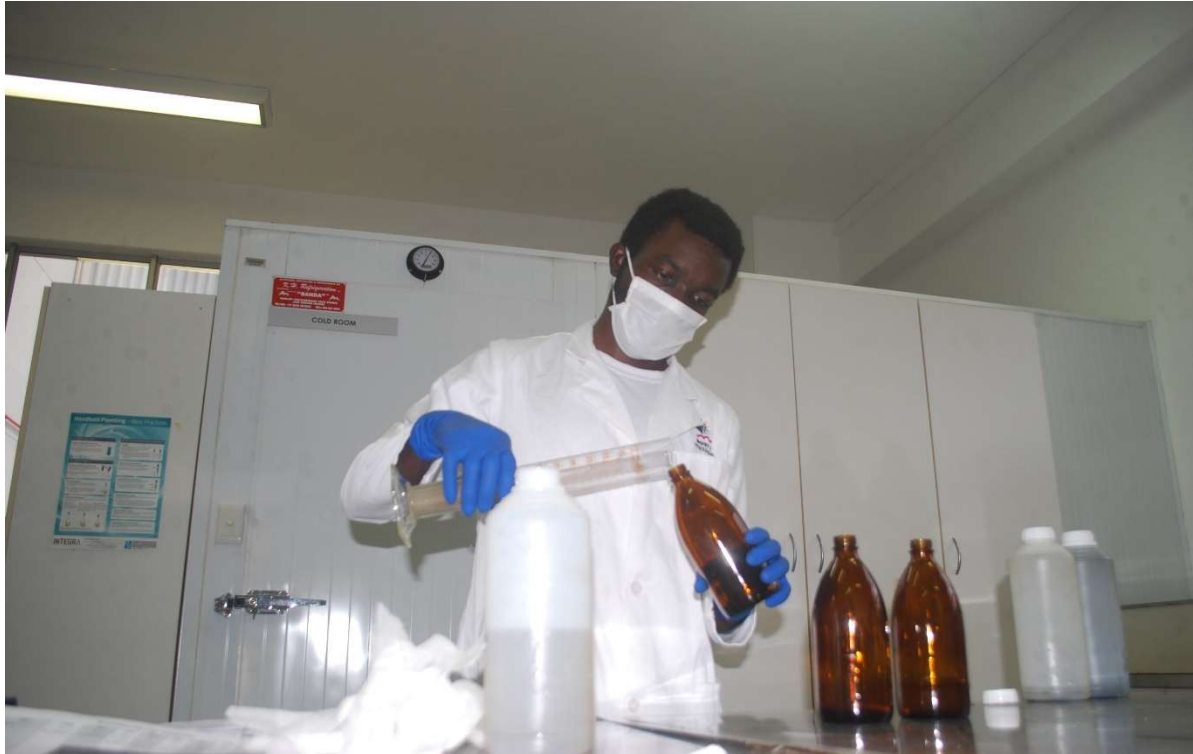
Figure 3-33: Wastewater sample being measured into BOD bottles
