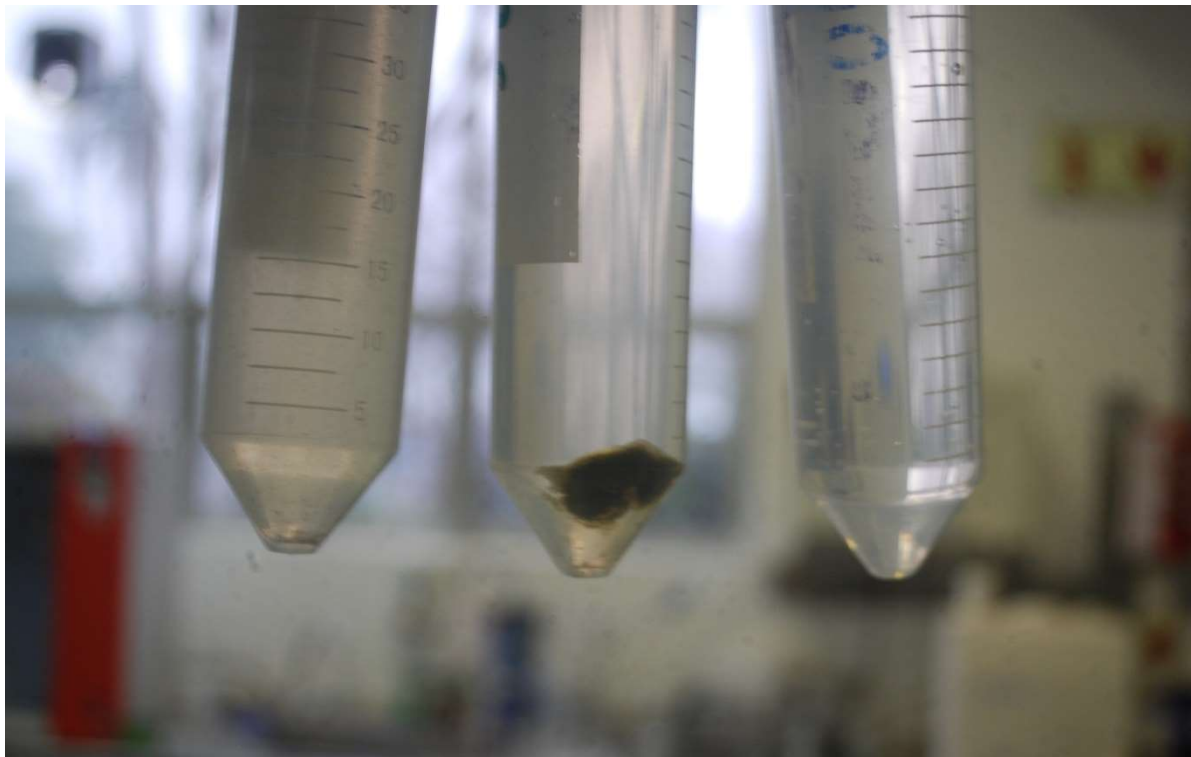
Figure 3-39: Wastewater sample in its raw state (left), after centrifugal separation (middle), and after microsieving (right)
