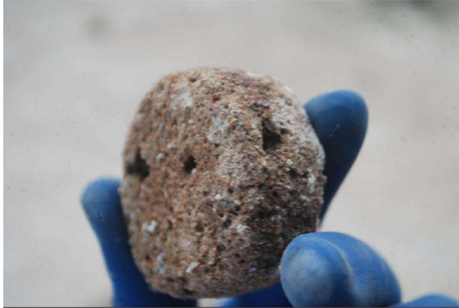
Figure 4-21: PCA m sample after 9-month exposure
