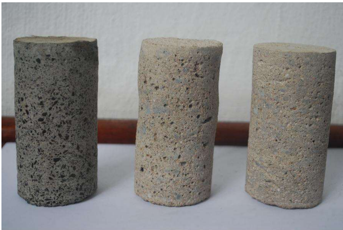
Figure 3-9: Cored mortar cylindrical samples, CAC m (left), PCA m (middle), PC m (right)
