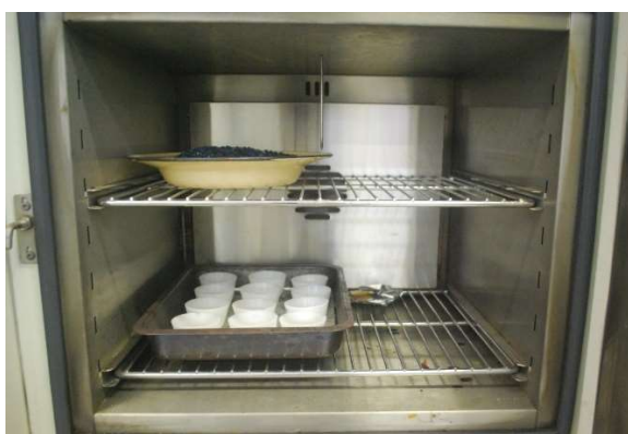
Figure 3-29: Wastewater sample being weighed (left) and placed inside the oven (right)
