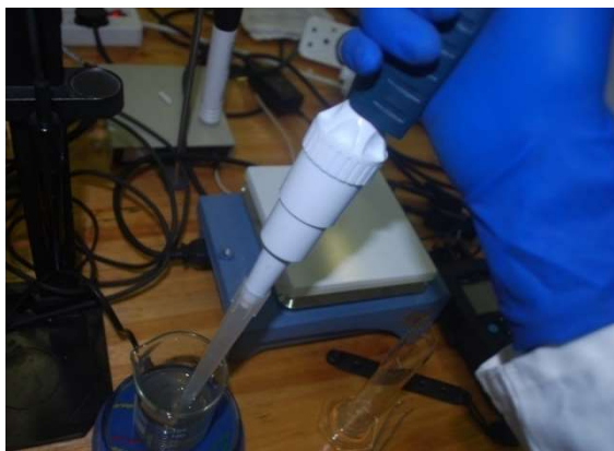
Figure 3-28: Measurement of wastewater sample into crucible
