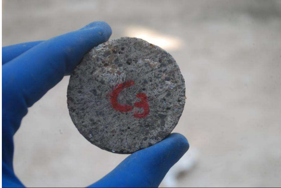
Figure 4-19: CAC m sample after 9-month exposure
