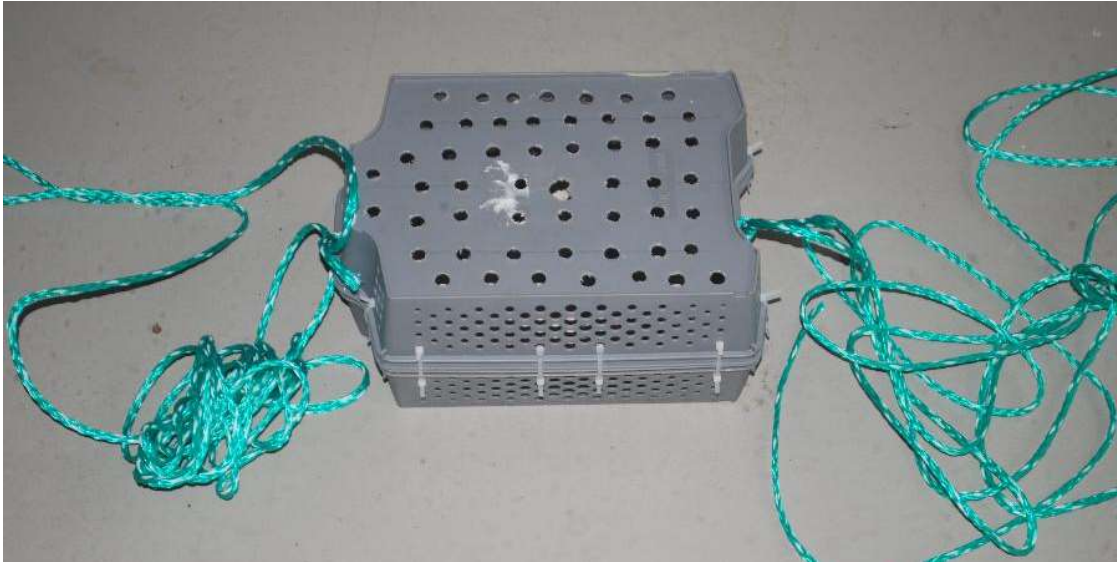
Figure 3-19: Prepared sample cage, ready to be transported to site
