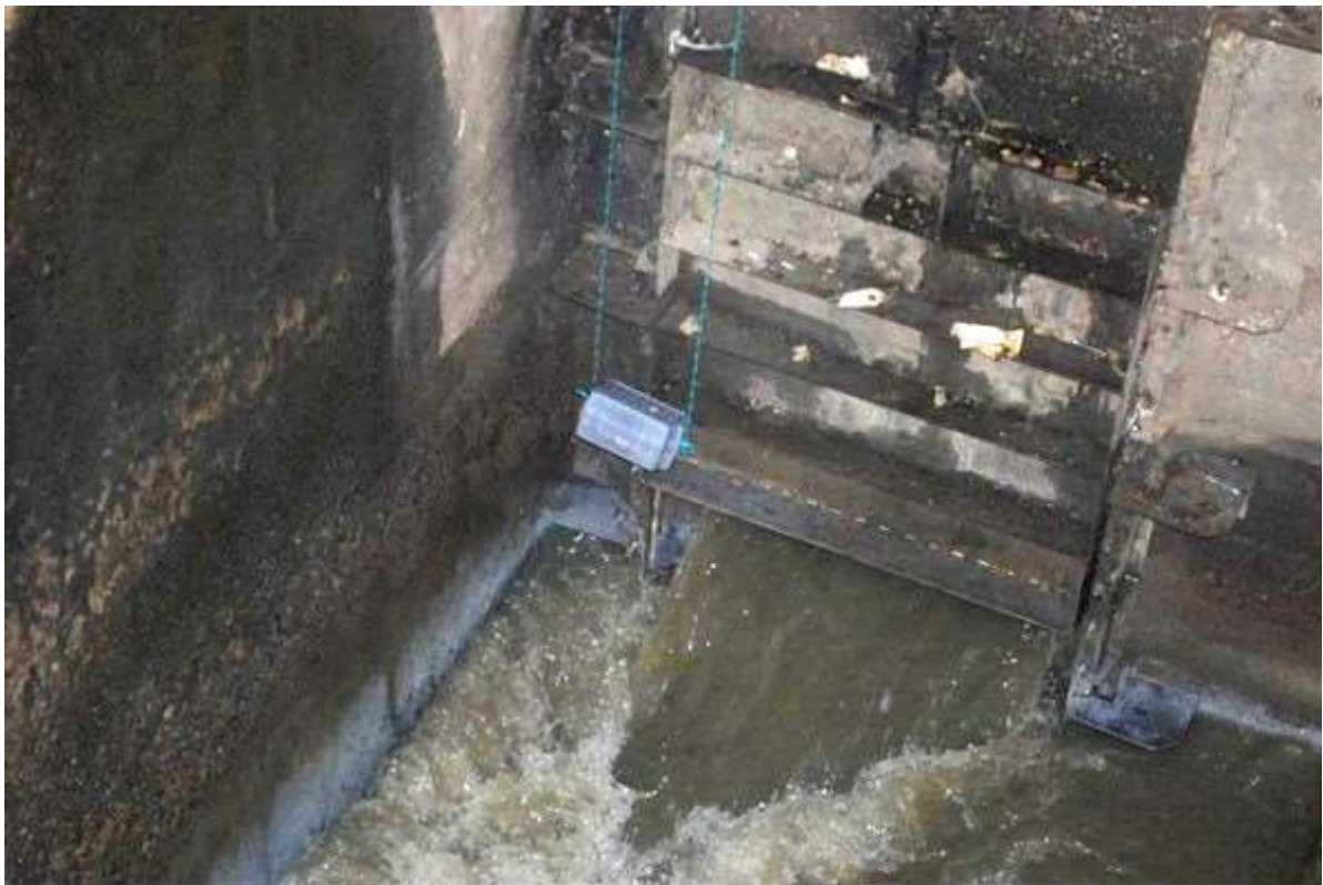
Figure 3-20: Suspended sample cage within the sewer environment
