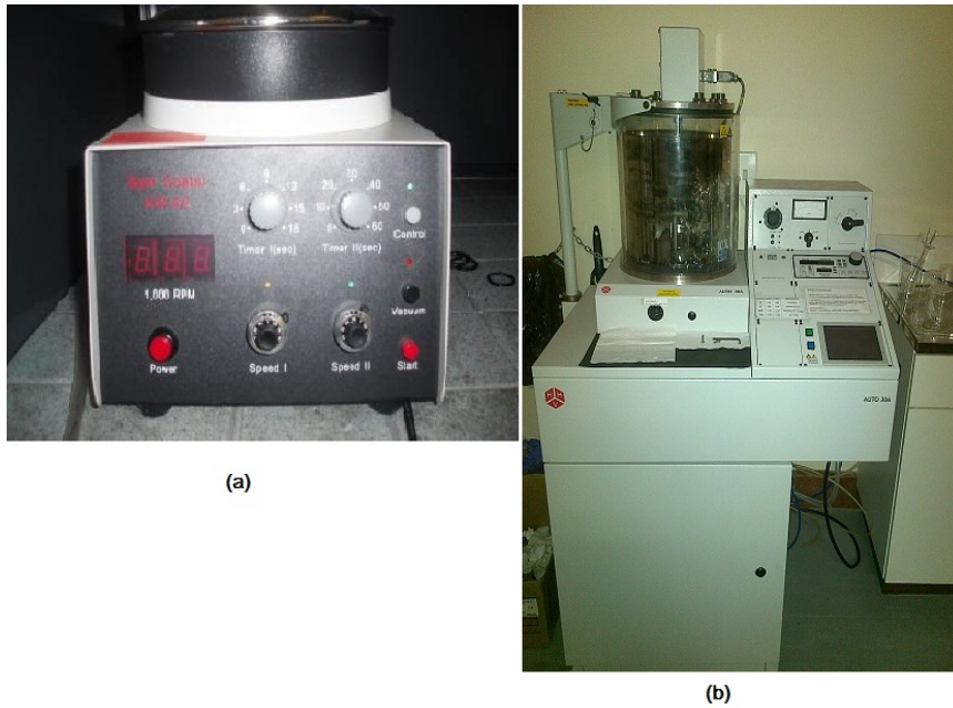
Figure 5.1: (a) PI-KEM LTD Spin Coater KW-4A used for spin coating and (b) Edward Auto 306 used for the deposition of LiF and Al.
