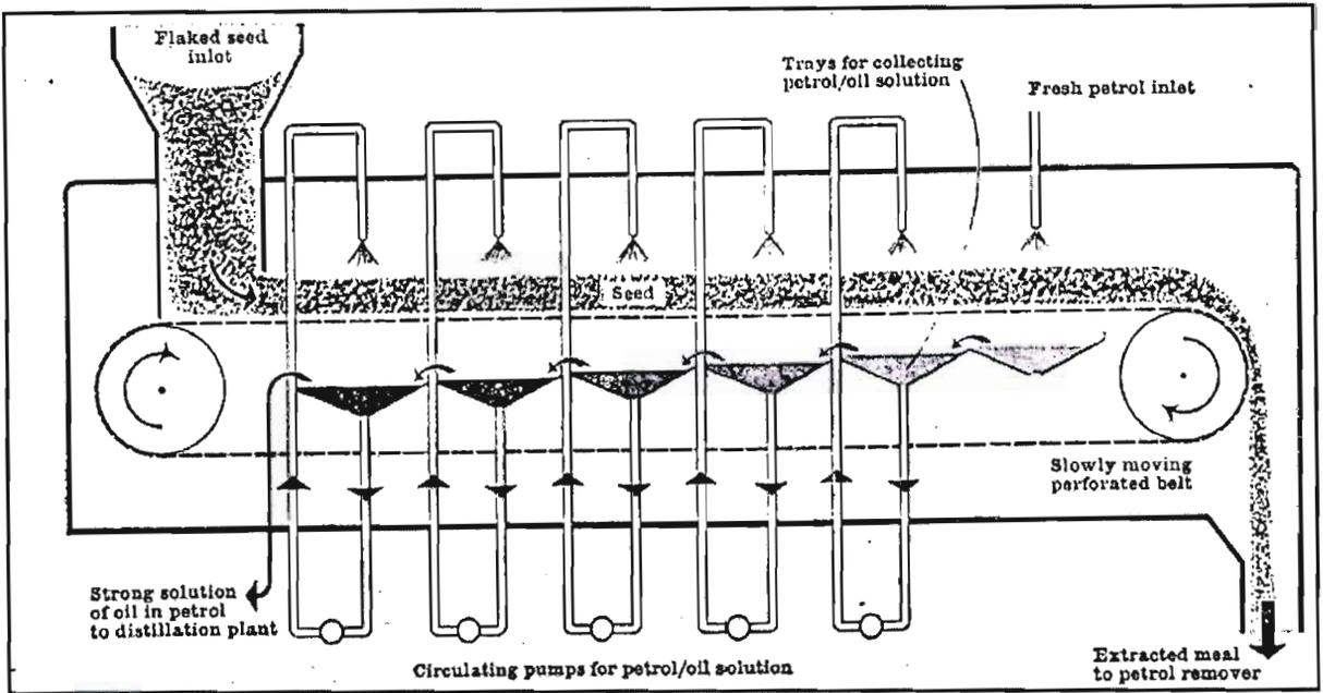
**Figure 3.3.** The solvent extraction process
