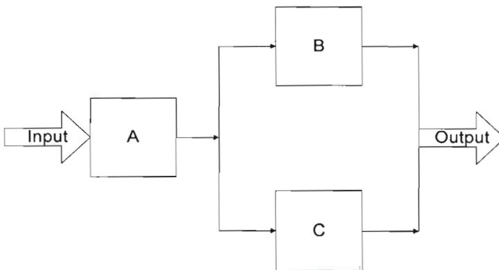
**Figure 2.3** A combined series-parallel network
