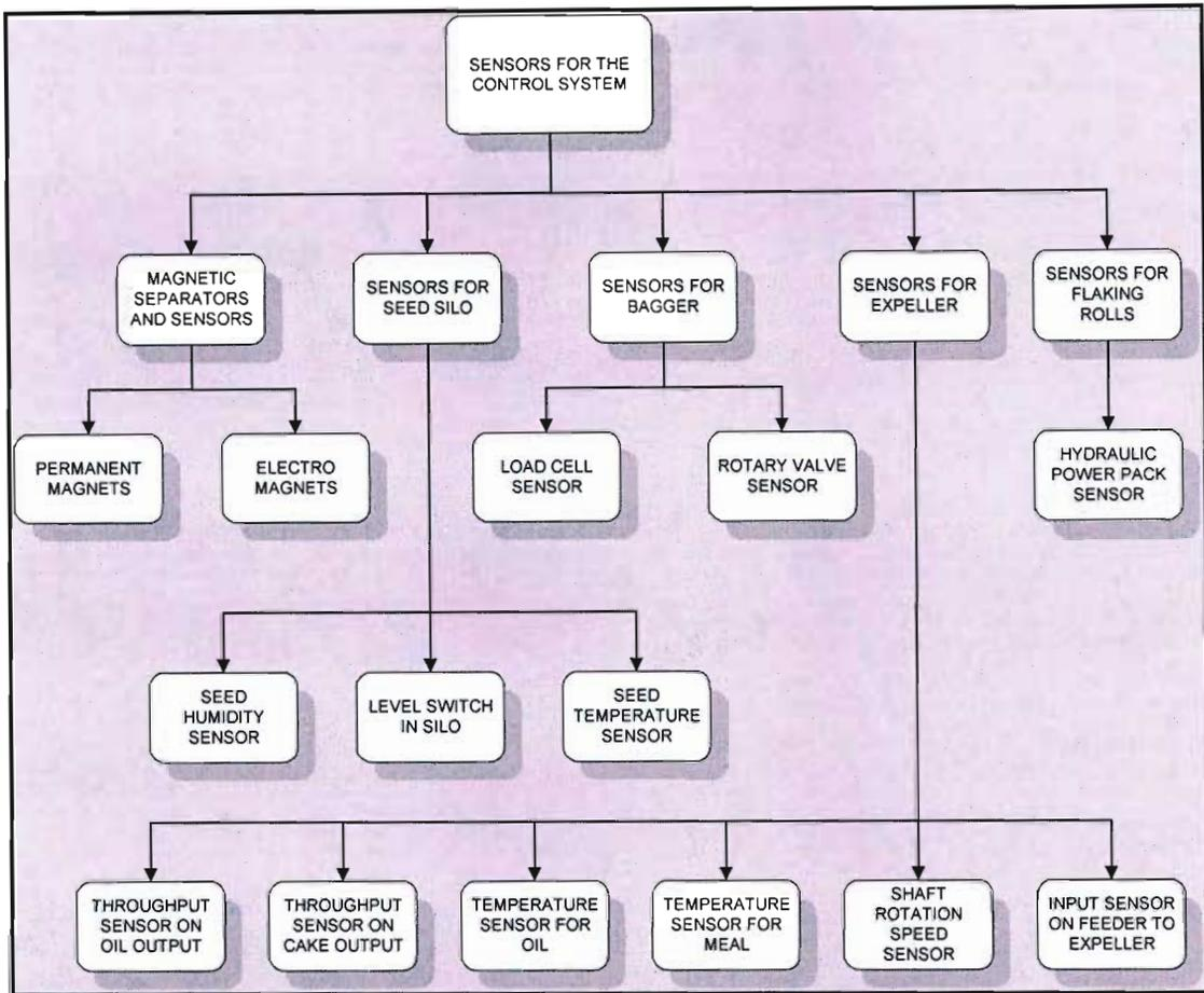
**Figure 4.6.** Product breakdown structure of the control system sensors
