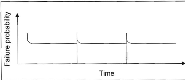
**Figure 4.15.** Failure pattern with traditional Time-Based maintenance
