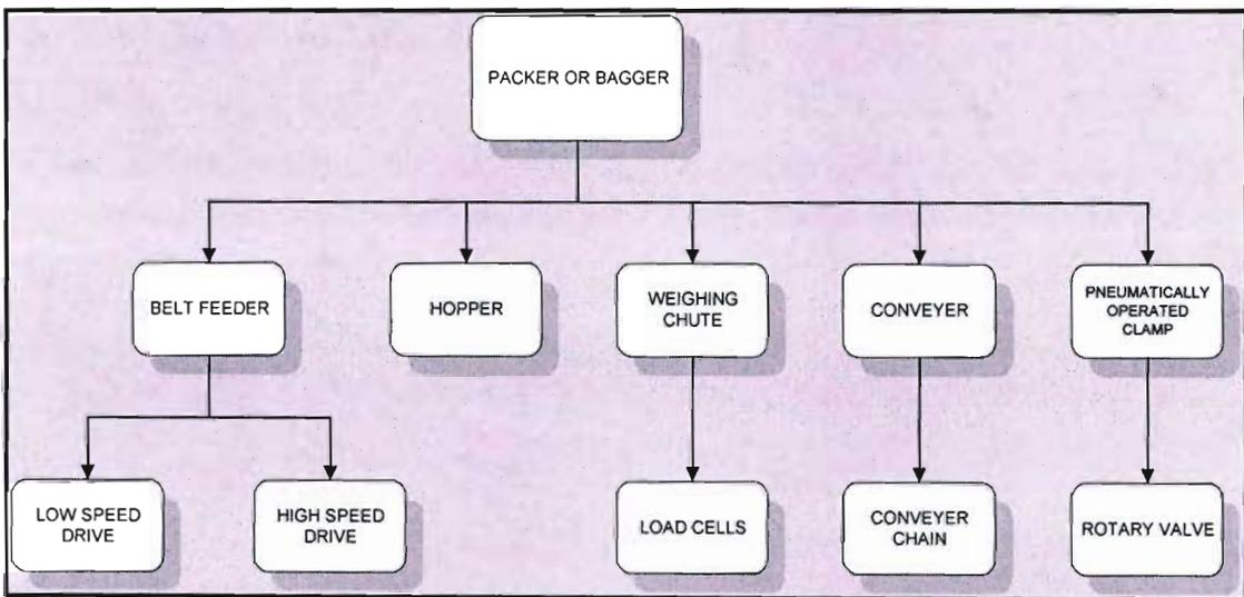
**Figure 4.5.** Product breakdown structure of the bagging machine
