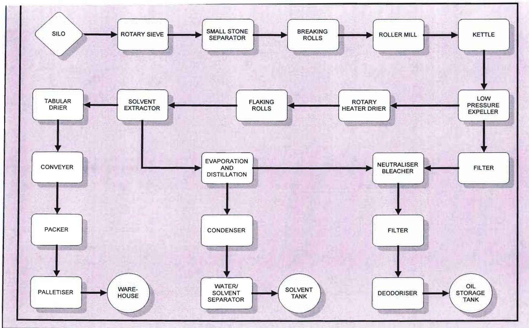
Figure 3.1: Oil Milling Process
