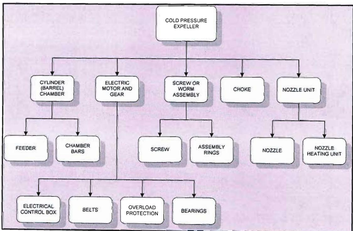
Figure 4.4. Product breakdown structure of the expeller
