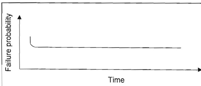
**Figure 4.16.** Failure pattern with condition based maintenance
