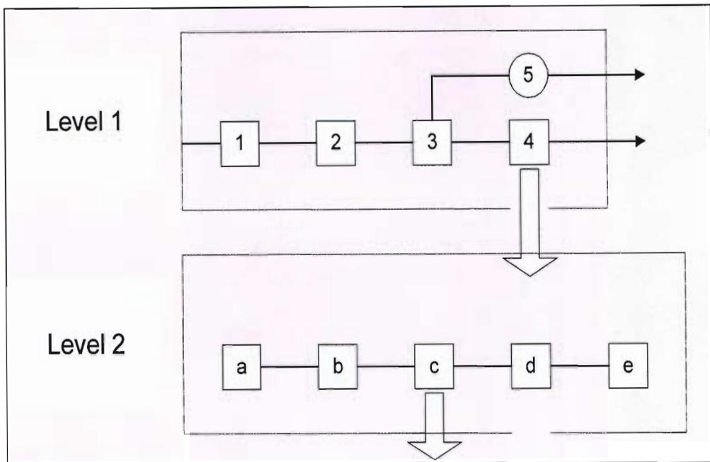
**Figure 2.5** Reliability block diagram method
