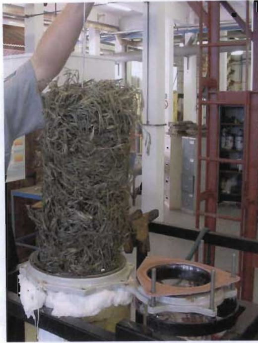
Figure 3.2 Removing charge from the test distillation apparatus.
