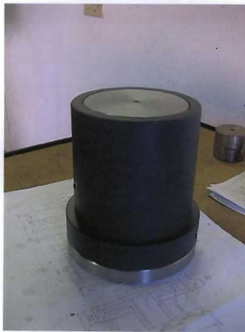
Figure 3.7 Nylatron GSM bush with bright steel shaft.
