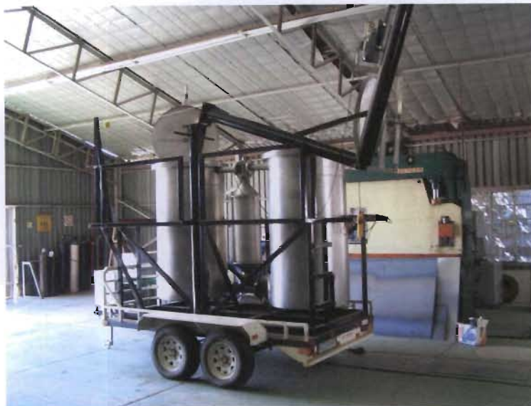
Figure 3.9 Mobile distillation unit with the crane in the transporting position.
