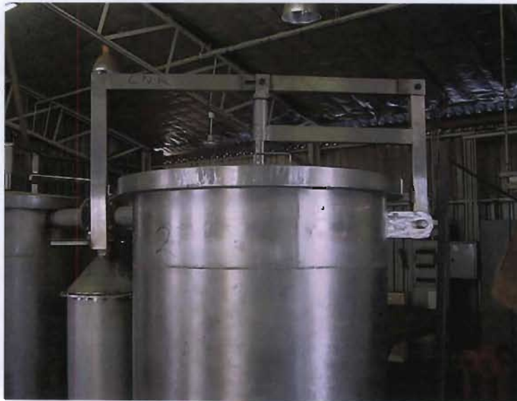
Figure 3.6 Charge vessel lid with opening mechanism.
