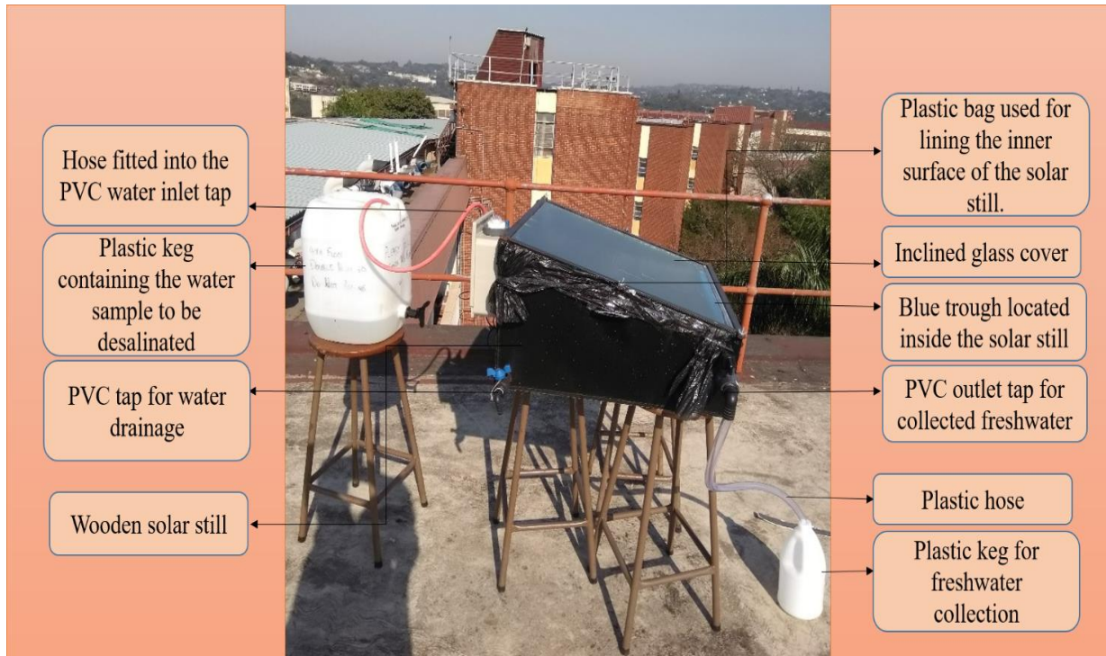
Figure 3.1: Set-up of a solar still prototype capturing radiant solar energy on a roof top
