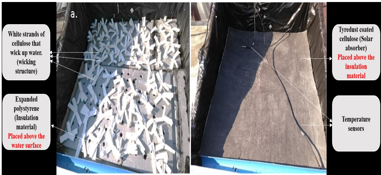
Figure 3.4: Image of the development of the evaporation structure in a solar still showing (a) insulator and wicking structure made of cellulose. (b) solar absorber placed on the wicking structure and temperature sensors.
