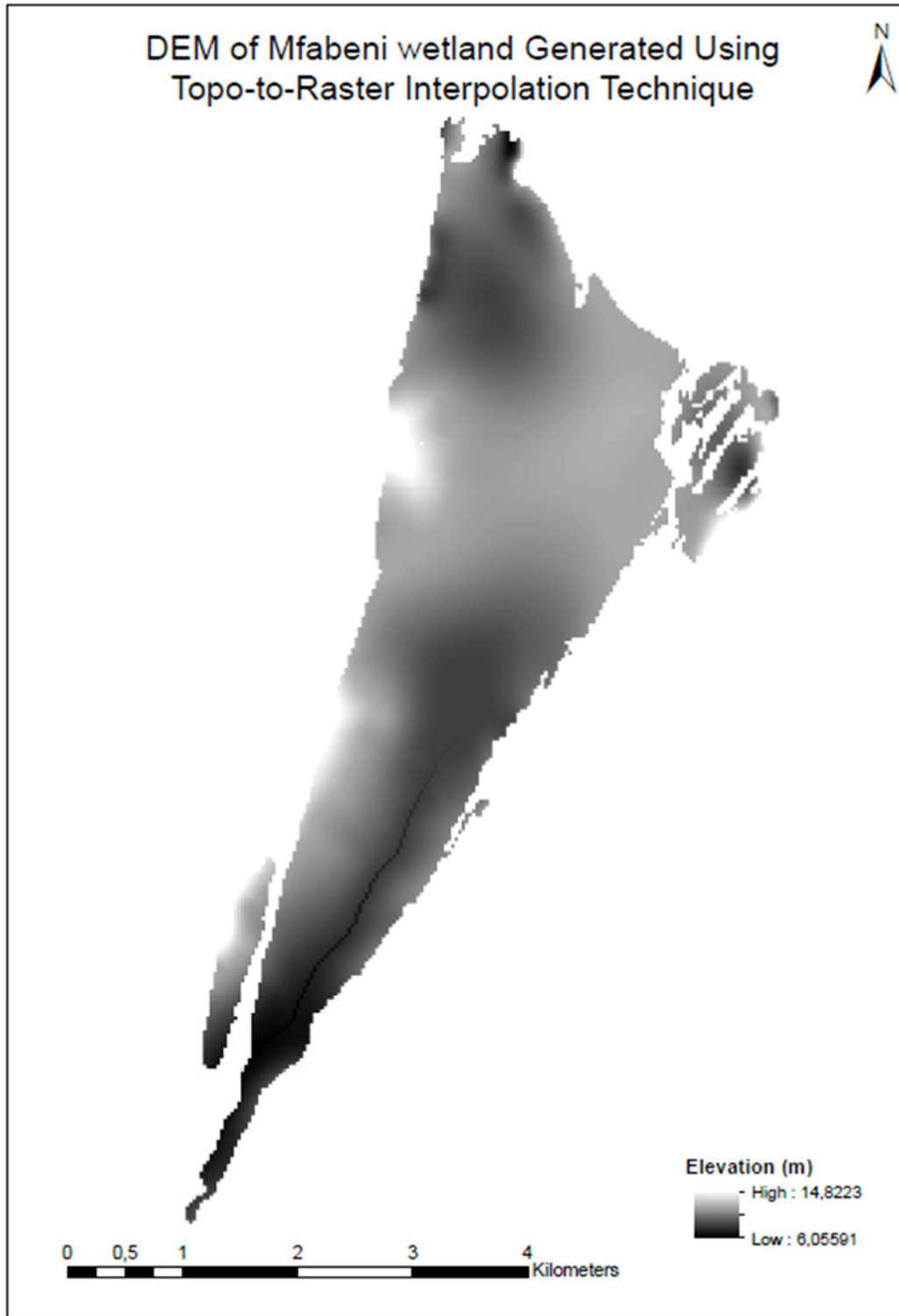
Figure 6.19: DEM of Mfabeni wetland Generated Using Topo-to-Raster Interpolation Technique
