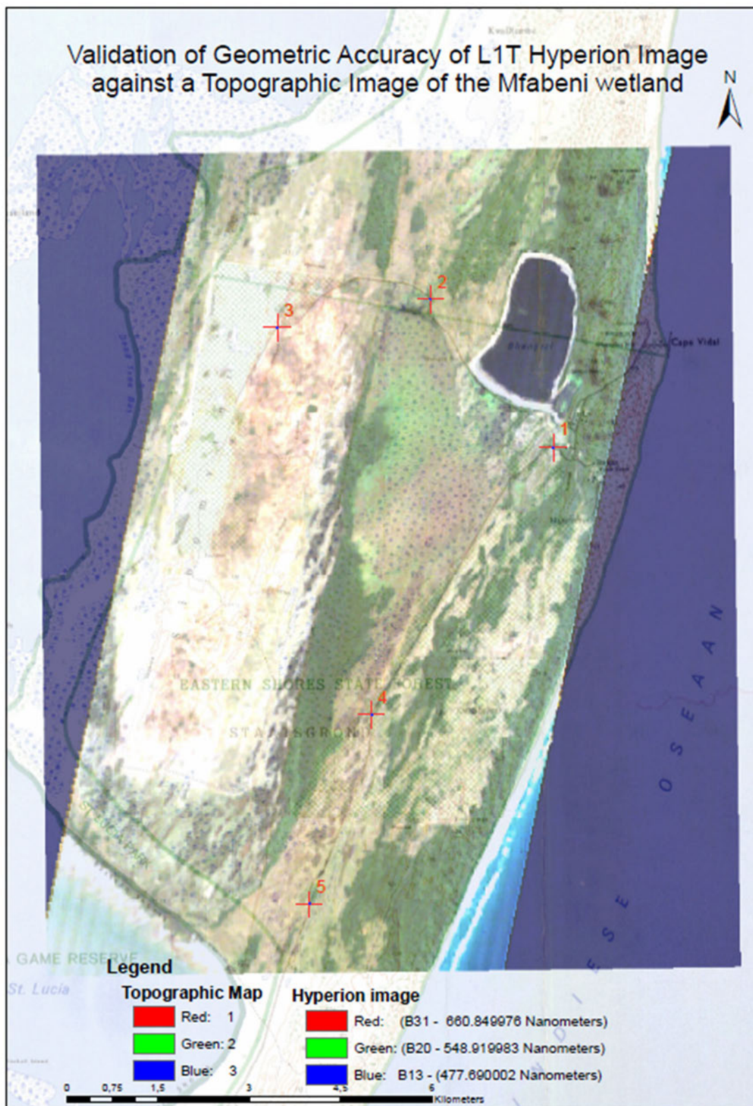
Figure 5.8: Hyperion image superimposed over the Topographic map of the Mfabeni wetland showing checkpoints used to validate the geometric accuracy of the L1T Hyperion image.
