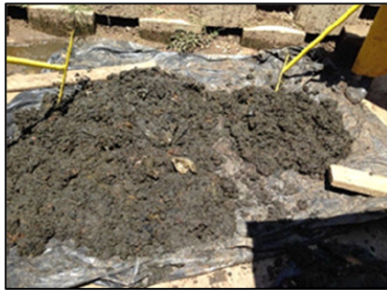
Figure 3.2: Screening of the UDDT sludge using rakes
