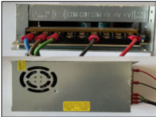
Figure 8: AC to DC Power Supply
