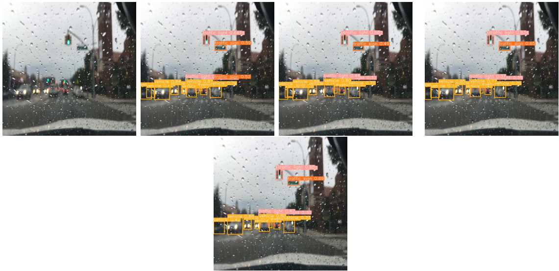
Figure 4.8: Detection results in the rain frame2:yolov8, frame3:GAM, frame4:CBAM, Frame5:ECA
