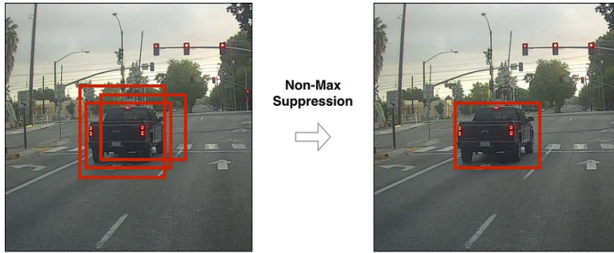
Figure 2.10: Before and after application of NMS
