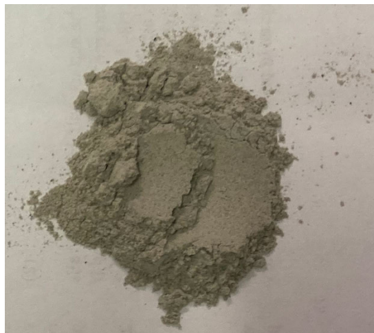
Photograph 3.5: Light fly ash sample obtained from Majuba power station
