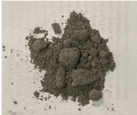
Photograph 3.4: Dark fly ash sample obtained from Camden power station
