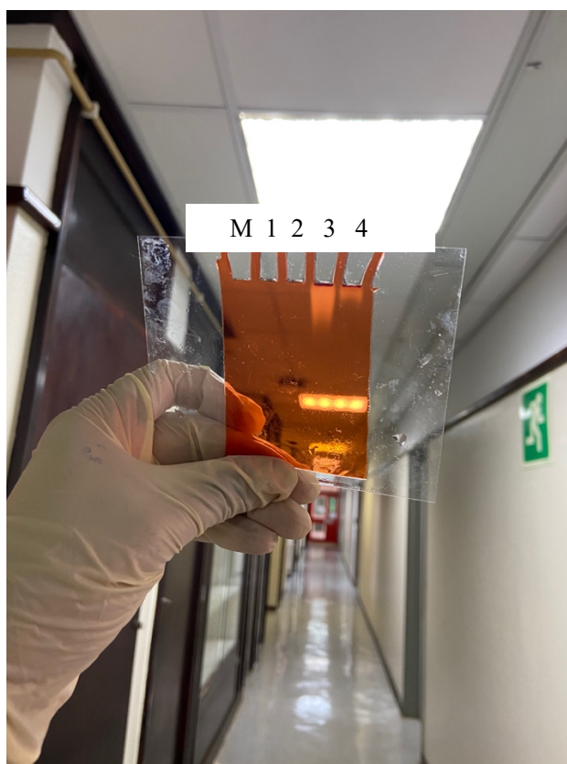
Figure 4: Original native-substrate PAGE gel (stained) image representing lanes M: Molecular weight marker (Thermoscientific, USA), 1: crude, (not concentrated), 2: purified 50% fraction (not concentrated), 3: crude (concentrated), and 4: purified 50% fraction showing zones of clearance. Lane 4 was cropped for the manuscript and is represented in chapter three, figure 3.9b, Lane 2.
