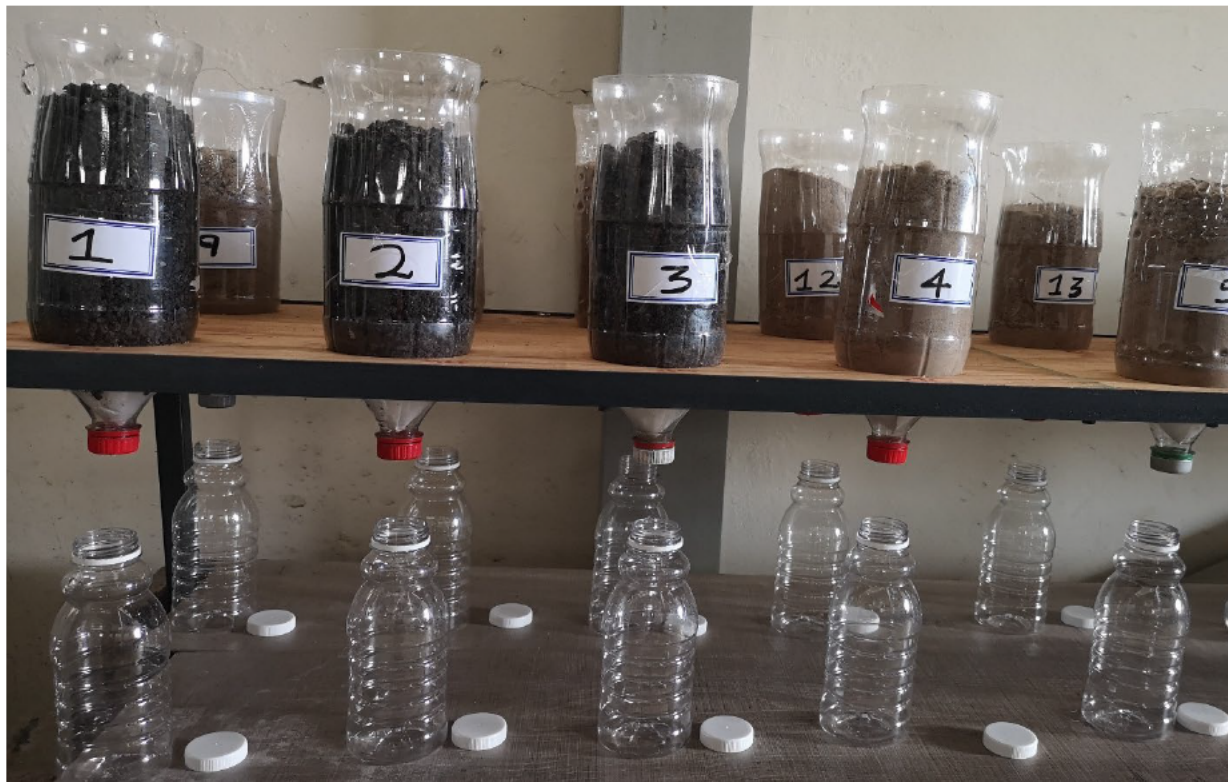
Figure 3. 12: Column Study Set Up Using Cut 2L Bottles in An Inverted Position.
