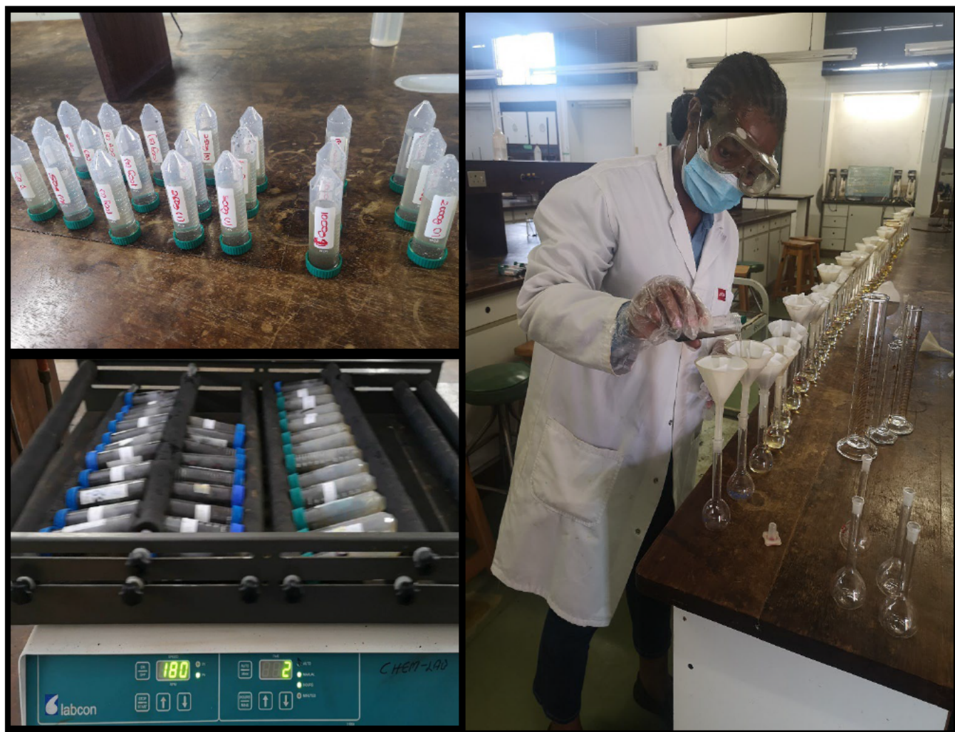
Figure 3. 4: sludge samples suspended in sorption solution, being shaken and filtered for analysis.
