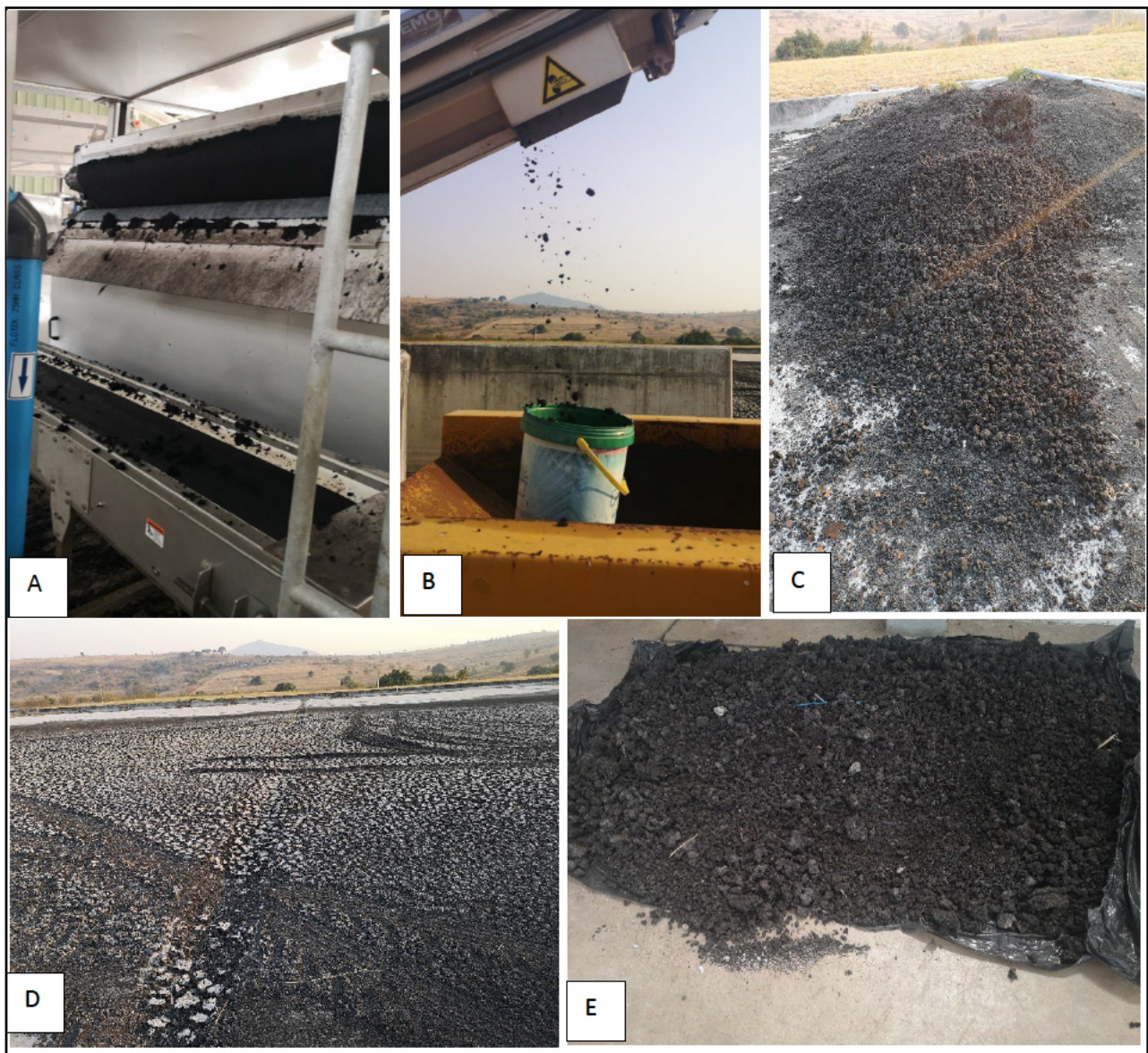
Figure 3. 2: A: Pressed sludge; B: Pressed wet sludge (August 2021); C: Air dried Sludge (June 2021); D: Air dried sludge (January 2021); E: Air dried sludge (August 2021)
