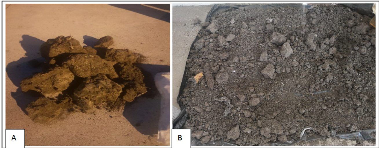
Figure 3. 3: A: Sampled domestic sludge – Nhlambeni WWTP; B: Sampled industrial sludge - Matsapha WTP
