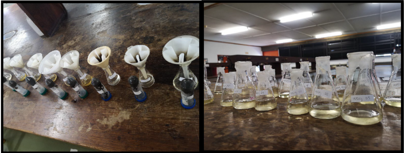
Figure 3. 5: TCLP samples ready for heavy metals analysis using ICP-OES
