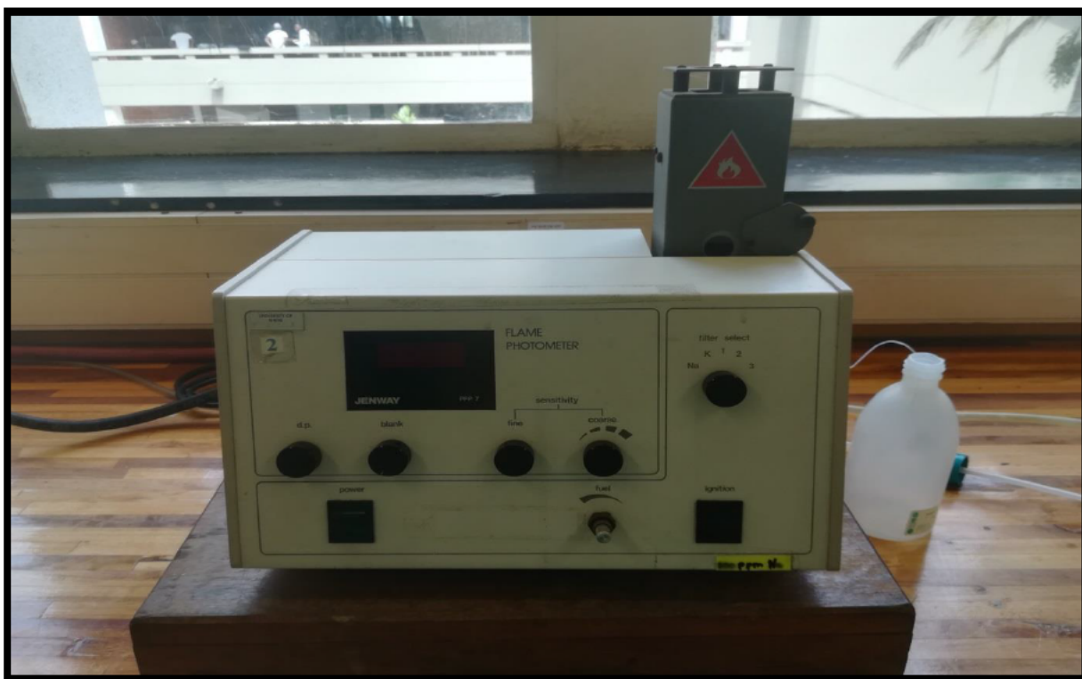
Figure 4.7. Flame photometer was used for sodium and potassium analysis of leachate and river water analysis.
