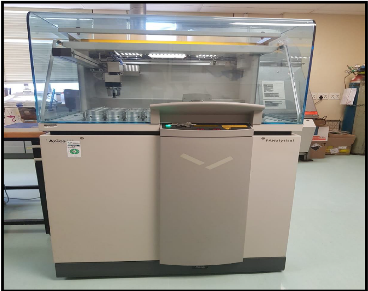
Figure 4.1. The PAN analytical Axios Wavelength Dispersive spectrometer used for whole rock element composition determination (CAF, 2021).
