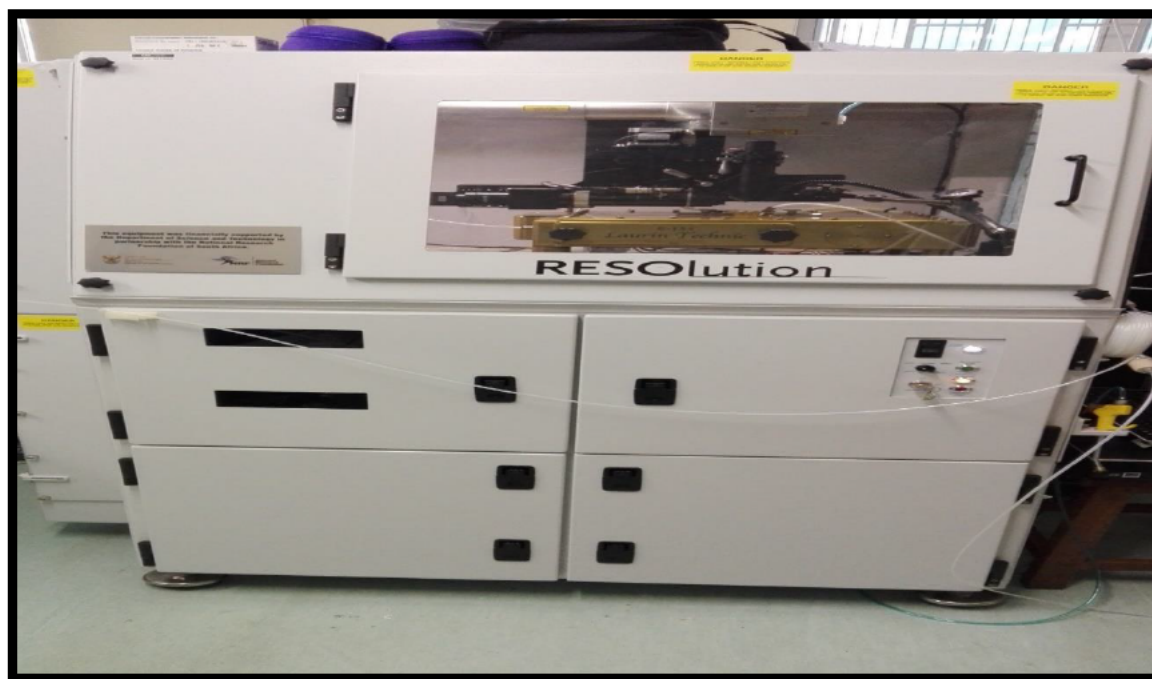
Figure 4.2. A Resolution 193nm Excimer laser from Applied Spectra connected to an Agilent 7700 Q ICP-MS (CAF, 2021).
