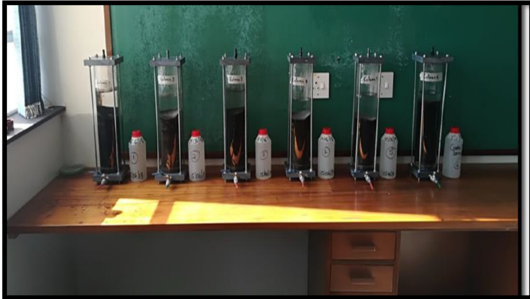
Figure 4: Humidity leach columns for the kinetic testing with weekly leachate.
