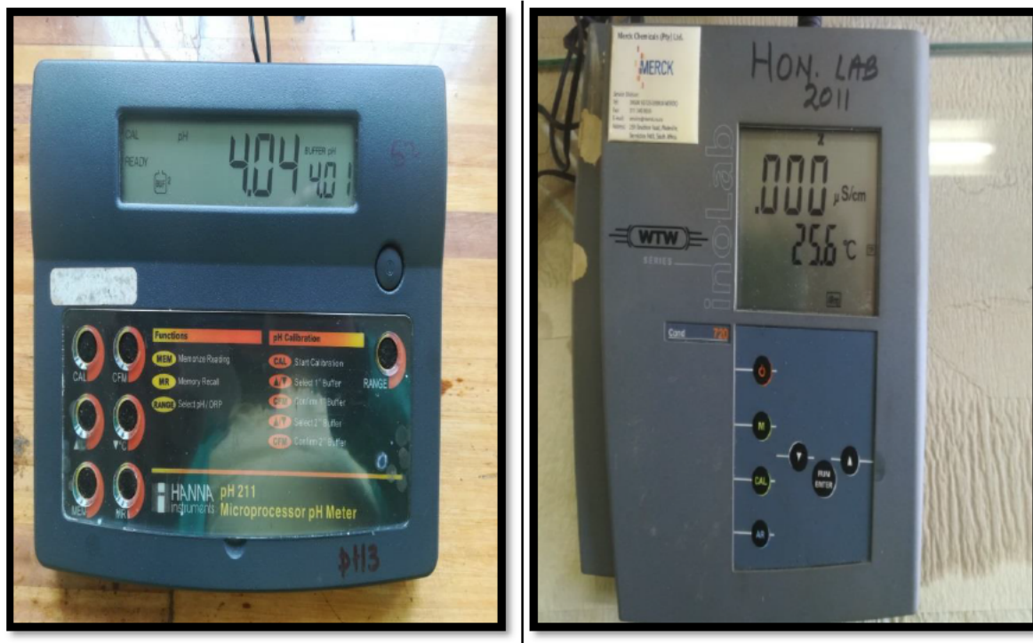
Figure 4.5. The Microprocessor pH meter (right) and the Inolab Con Level 1 Multiparameter Meter (left) were used in the measurements.
