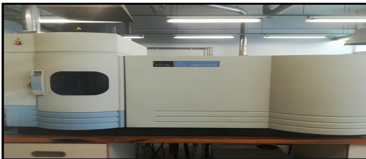
Figure 4.6. Perkin Elmer 8300 DV Inductively Coupled Plasma Optical Emission Spectrometry (ICP-OES) for leachate and river water analysis.
