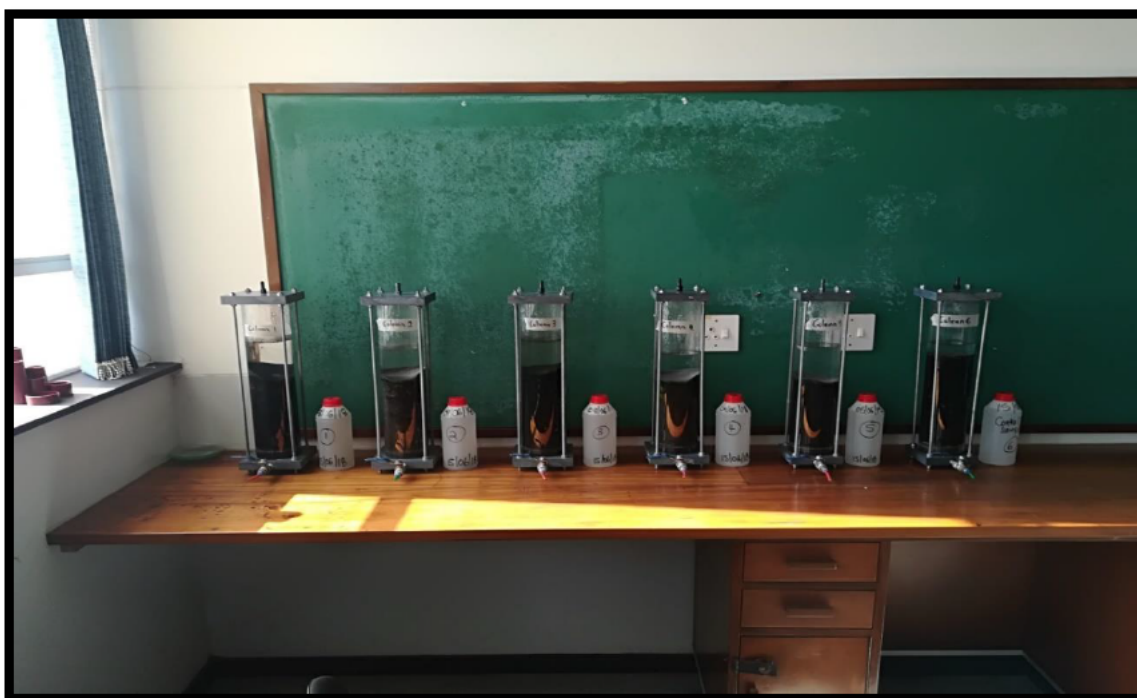
Figure 4.0. Humidity leach columns for the kinetic testing with weekly leachate.
