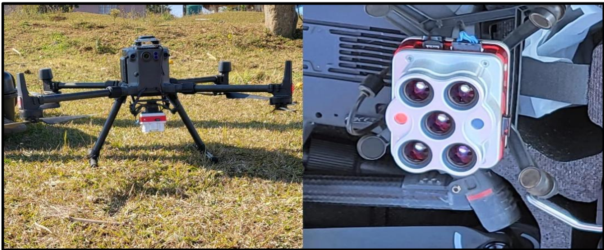
Figure 3.3 DJI Matrice 300 UAV platform and MicaSense Altum Multi-spectral camera
