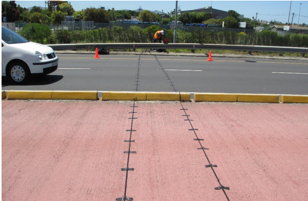
Figure 4. 9: Set-Up at Site SS003 with Installed Pneumatic Tubes and ATCs
