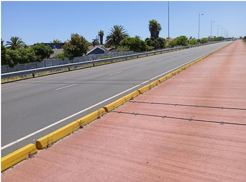
Figure 4. 5: Set-Up at Site SS002 with Installed Pneumatic Tubes and ATCs
