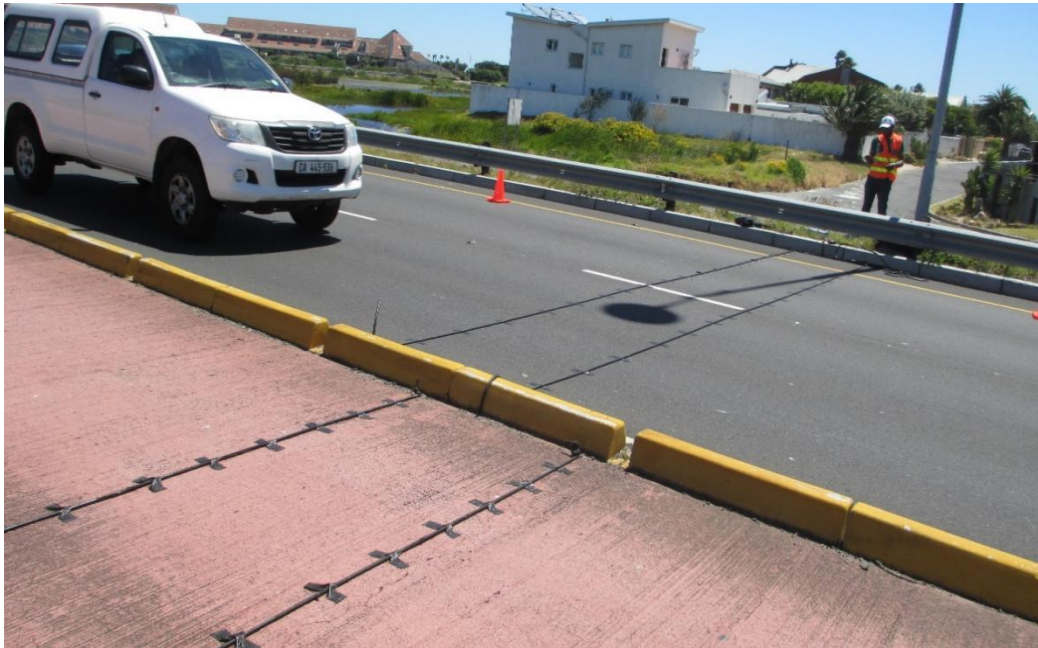
Figure 4. 13: Set-Up at Site SS004 with Installed Pneumatic Tubes and ATCs
