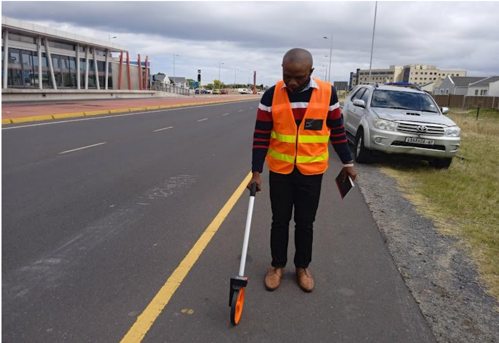
Researcher Measuring Roadway Segment Length
