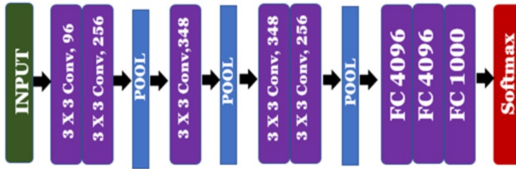
Fig. 6: ResNet Framework with 3 fully connected layers and one softmax function for multi-class problem
