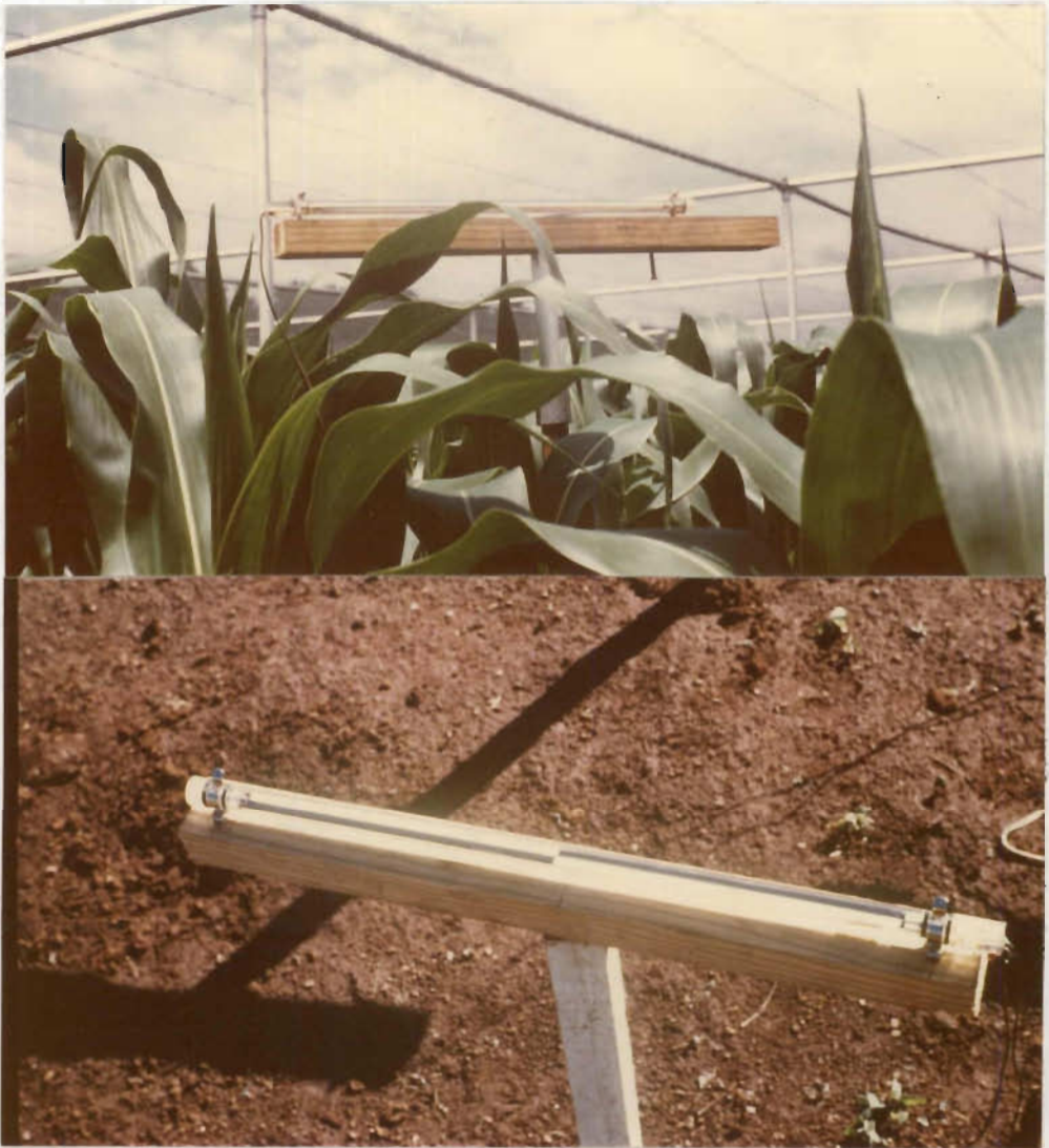
Plate 1.1: Tube solarimeters used to measure incoming solar radiant energy.
