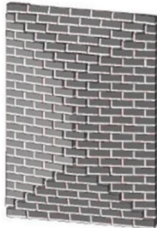
Figure 2. Out-of-plane failure pattern of a wall subjected to blast loading.
