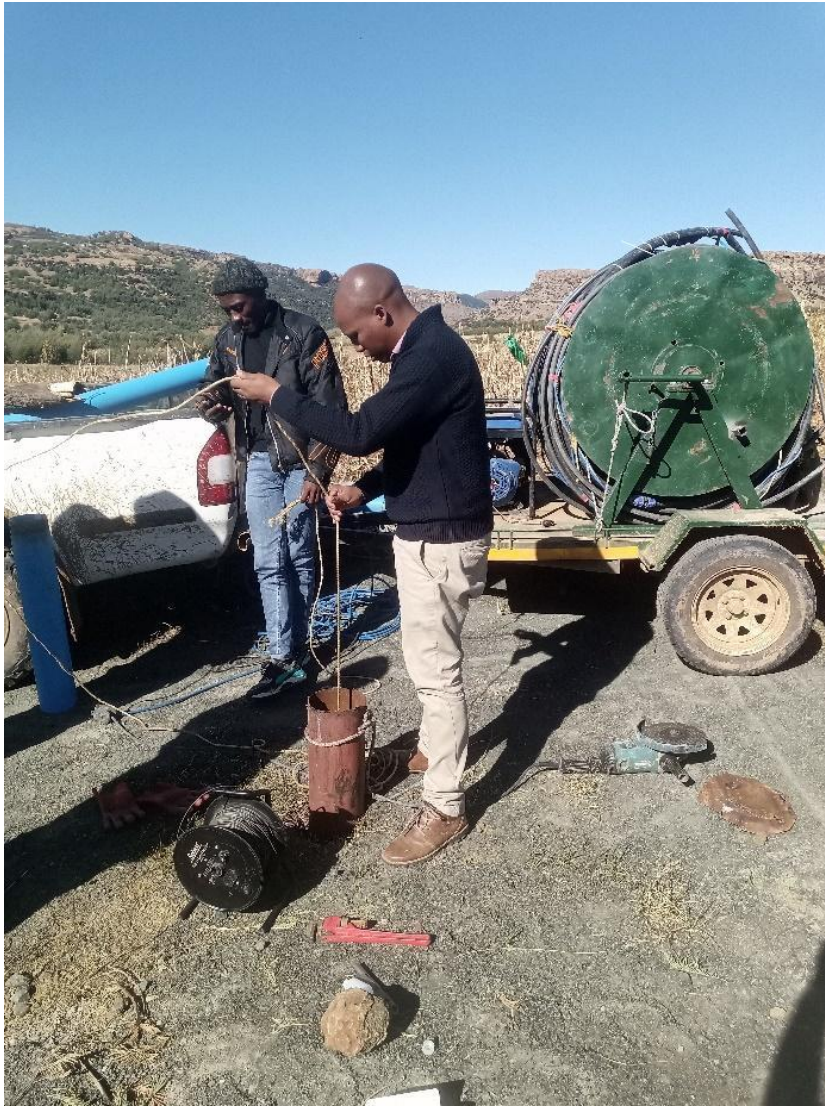
Figure 4.6 Sampling of borehole water using a bailer, illustrating a manual method for groundwater collection during field investigations.
